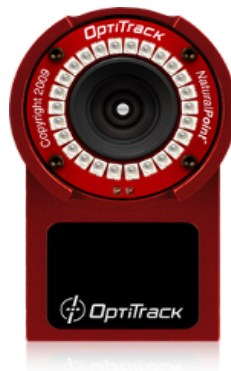
Figure 2.14: V100:R2 camera used for measuring robots' states (NaturalPoint, Inc., 2016)
