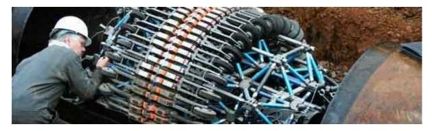
Figure 2-1.MFL equipment inserted inside the pipe (adopted from www.emtek.us)
