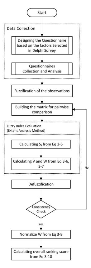
Figure 3-3.Flowchart for FAHP method
