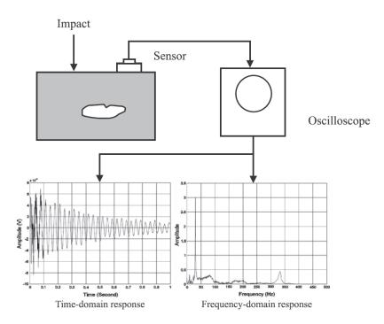
Figure 2-6.Basic principle of Impact echo (adopted from Liu & Kleiner, 2013)
