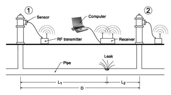
Figure 2-4.Principle of LeakfinderRT (adopted from Liu & Kleiner, 2013)
