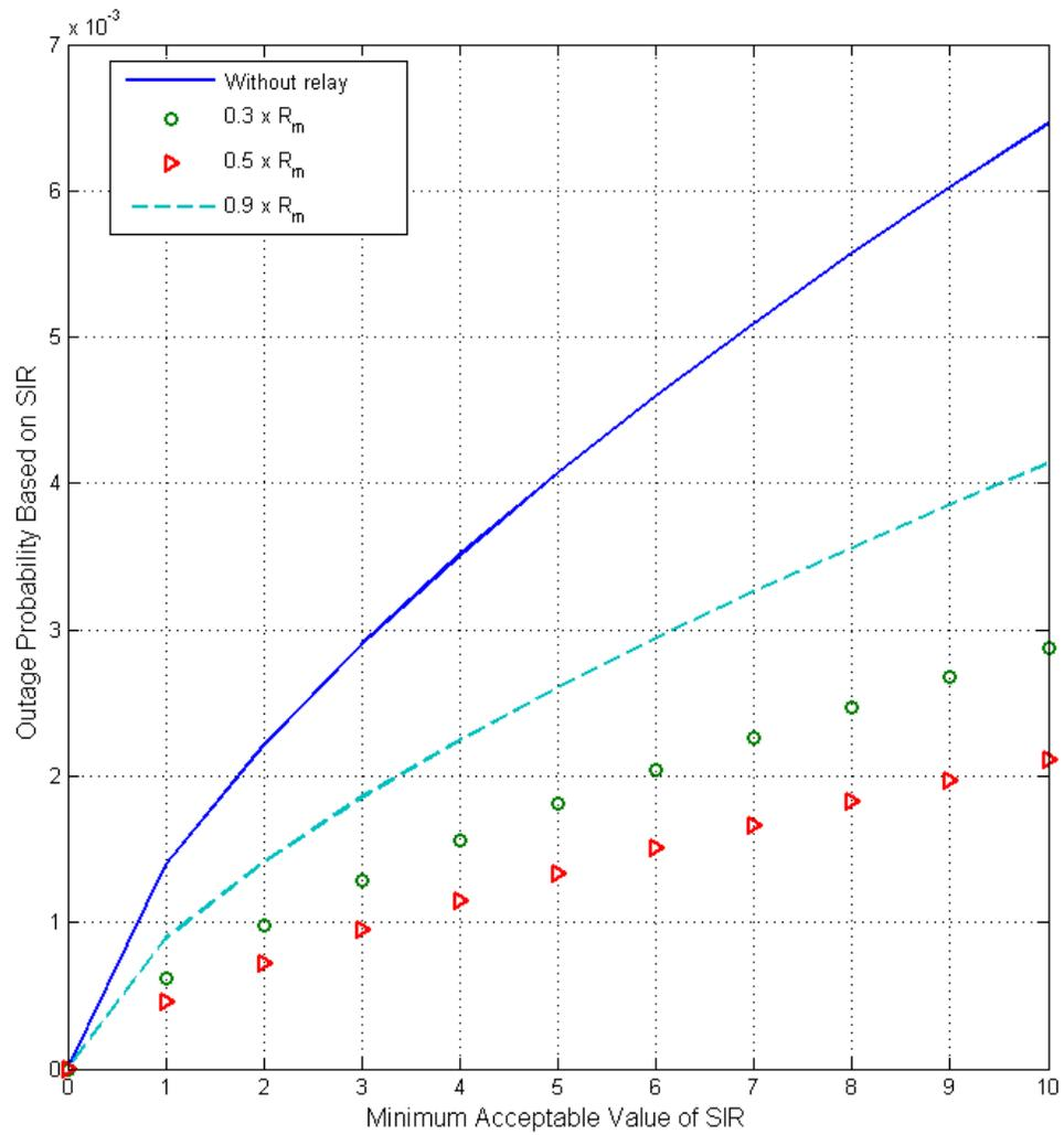
Figure 5.6: Outage probability based on SIR threshold for 6 relays located at  $0.3 \times R_m$ ,  $0.5 \times R_m$  and  $0.9 \times R_m$
