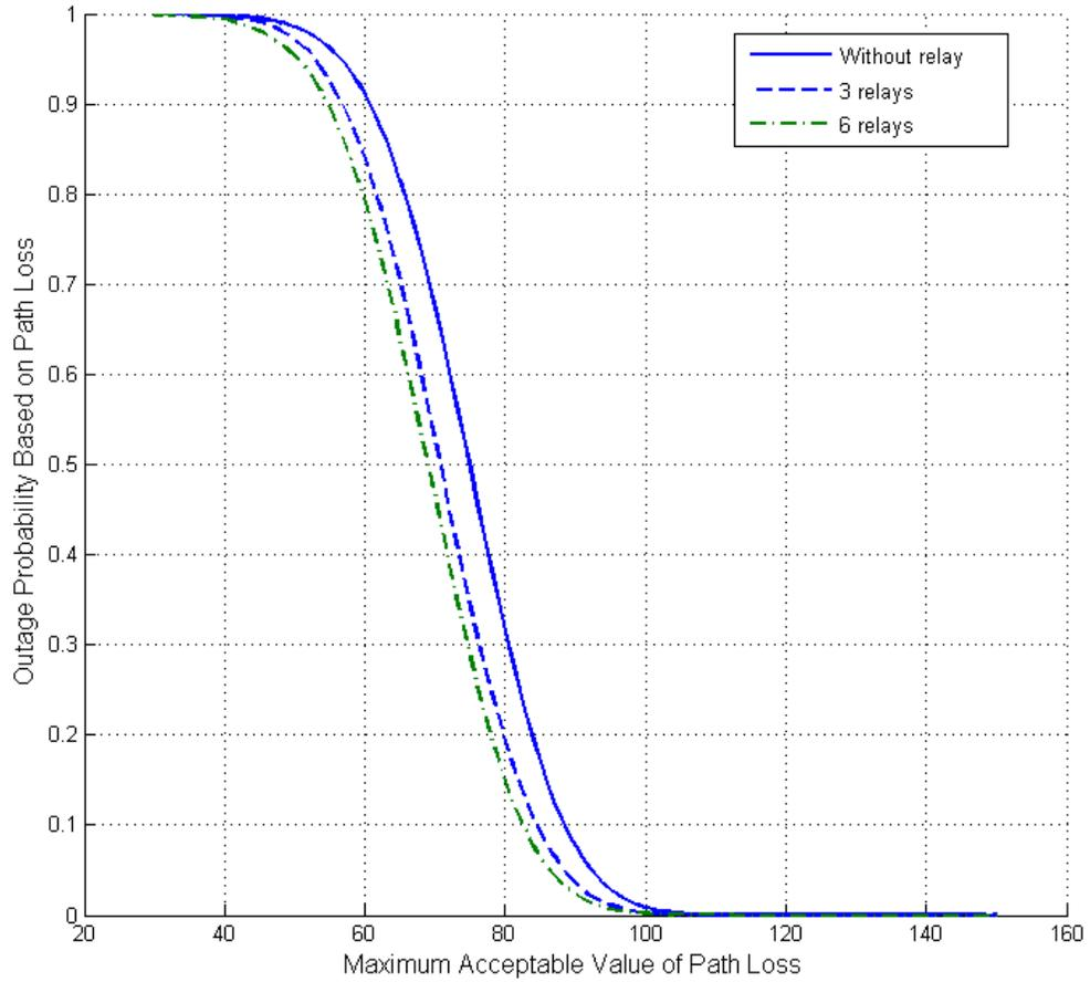
Figure 5.1: Outage probability based on PL threshold for different number of relays located at  $0.5 \times R_m$  from the BS
