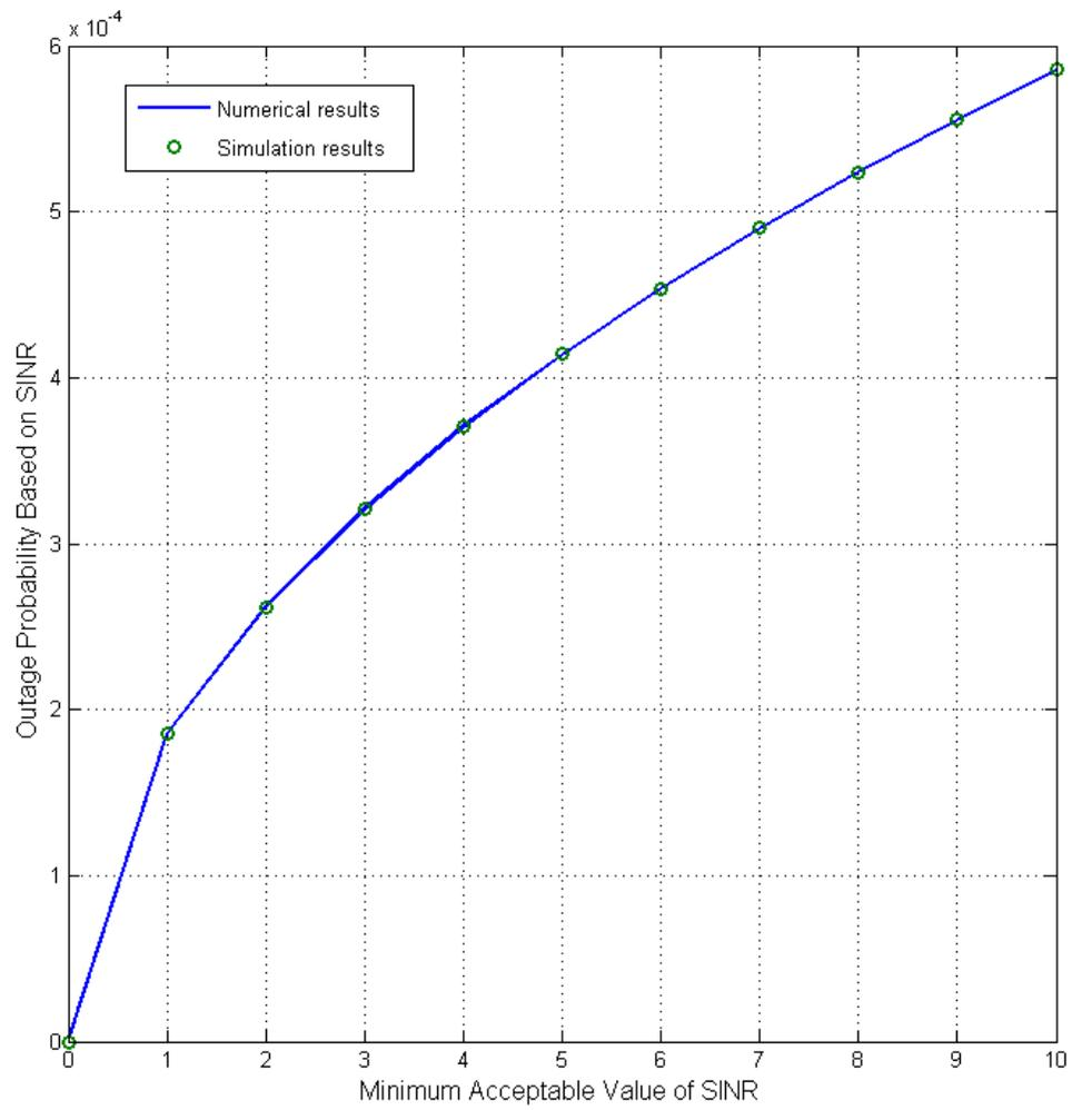
Figure 4.4: Outage probability based on SINR threshold in a circular cell
