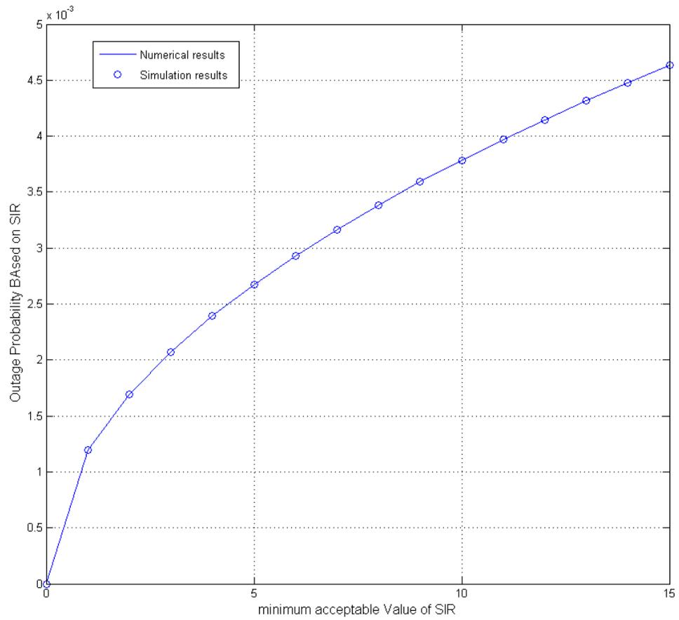
Figure 6.4: Outage probability based on SIR threshold for Gaussian distributed users in a circular cell
