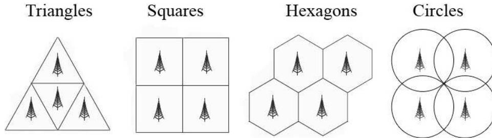
Figure 2.1: Circular cells versus cells with tessellating structures
