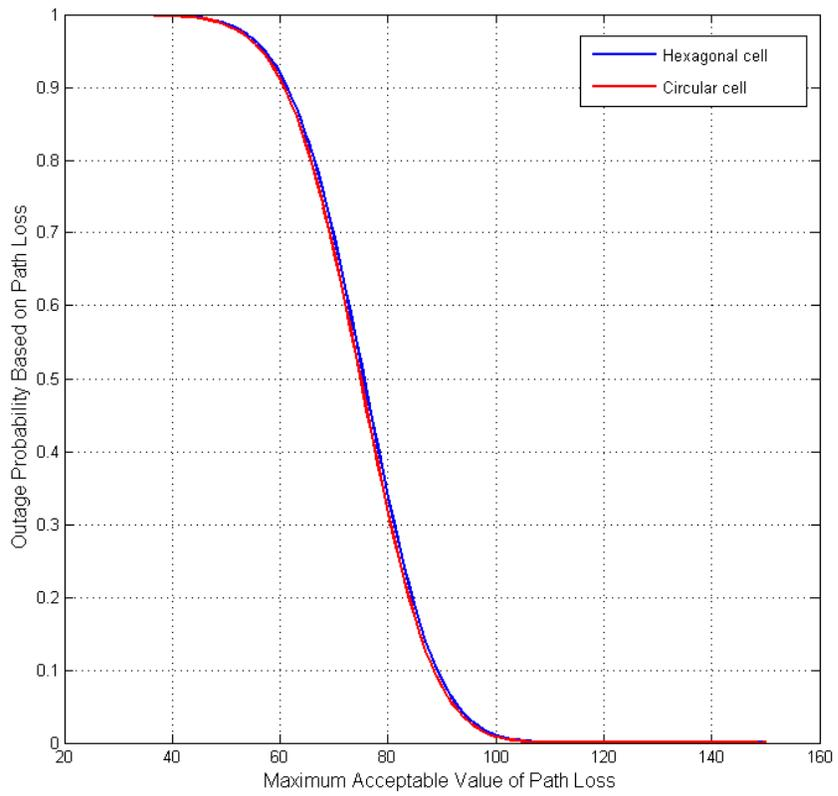
Figure A.2: Outage probability based on path loss for circular versus hexagonal cells
