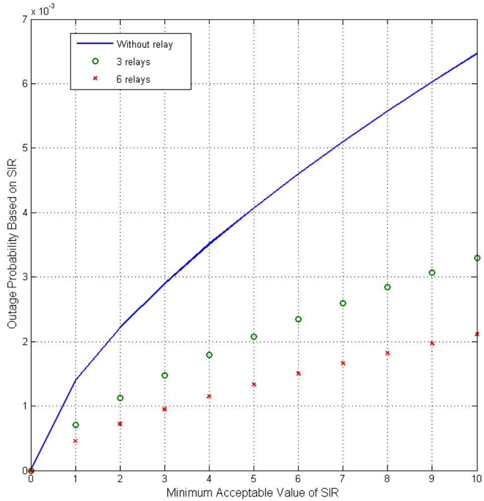
Figure 5.2: Outage probability based on SIR threshold for different number of relays located at  $0.5 \times R_m$  from the BS
