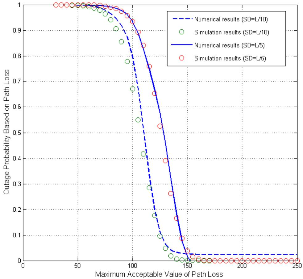
Figure 6.2: Outage probability based on PL threshold for different standard deviation of Gaussian distributed users in a circular cell
