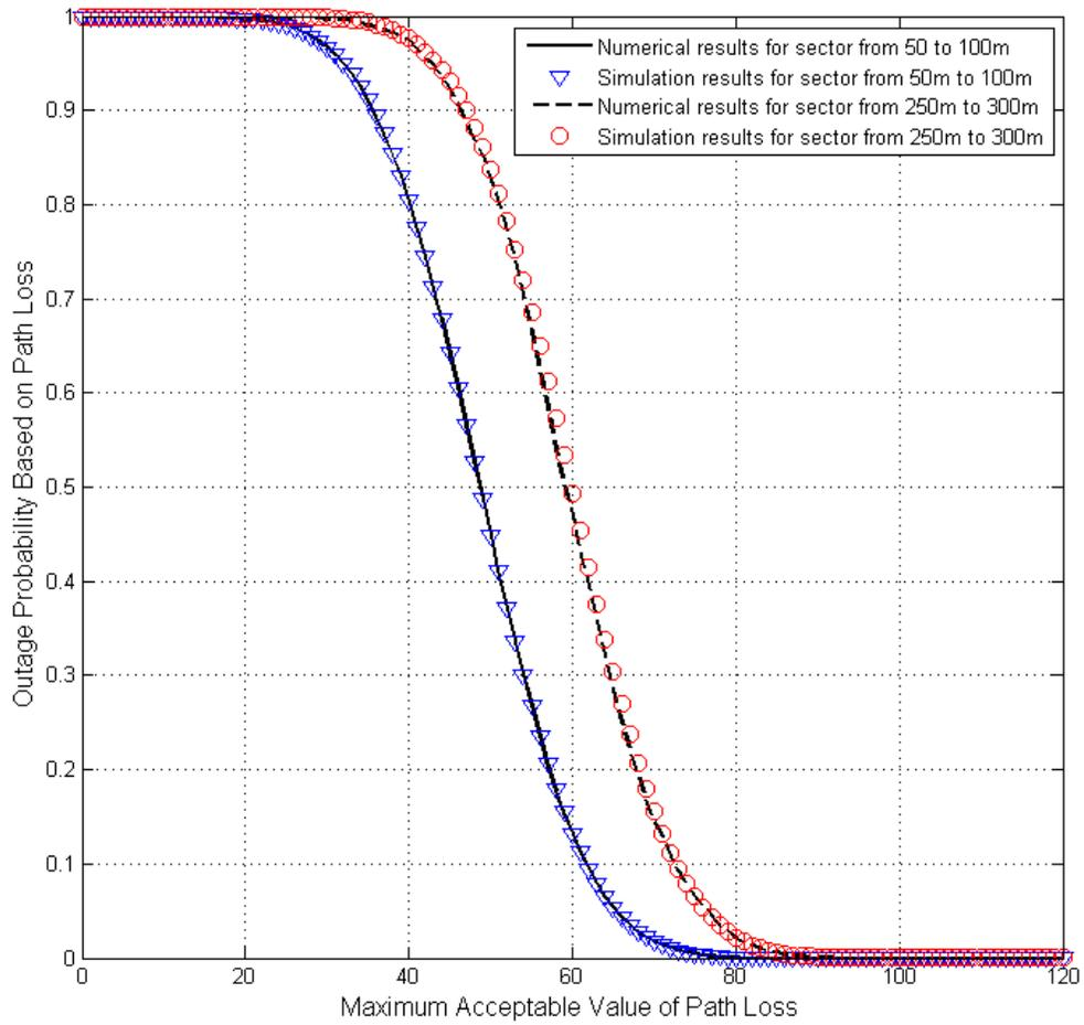
Figure A.4: Outage probability of different sectors of a circular cell based on PL
