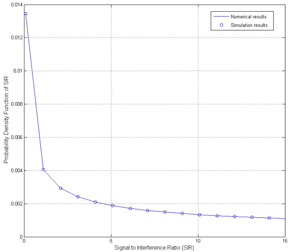
Figure 6.3: PDF of SIR for Gaussian distributed users in a circular cell for different cell sizes
