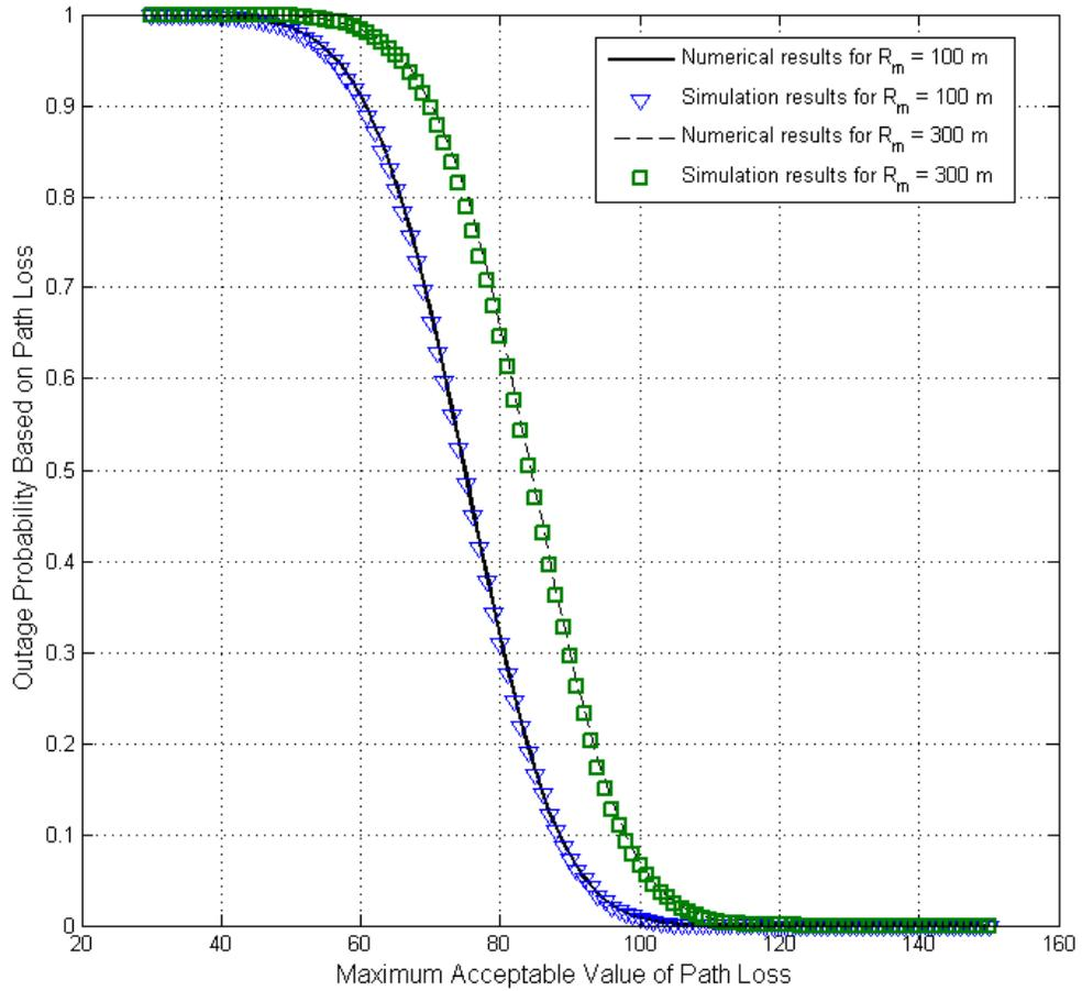
Figure 4.1: Outage probability based on PL threshold in a circular cell for different cell sizes
