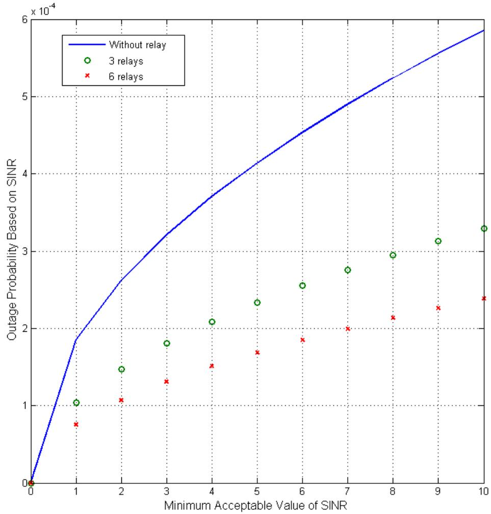
Figure 5.4: Outage probability based on SINR threshold for different number of relays located at  $0.5 \times R_m$  from the BS
