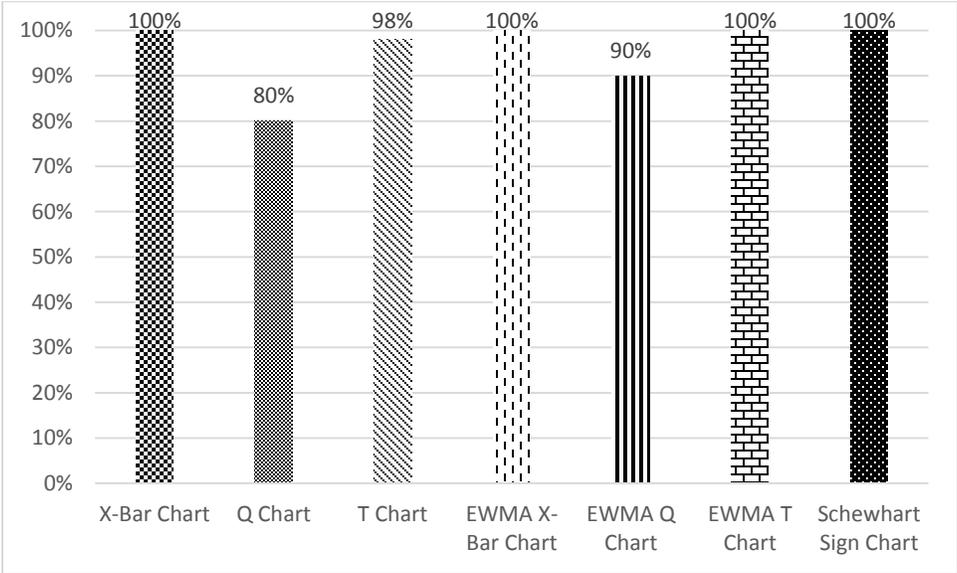
Figure 4.18 Success Rates of the Different Charts to Detect 1.5  $\sigma$  Mean Shift
