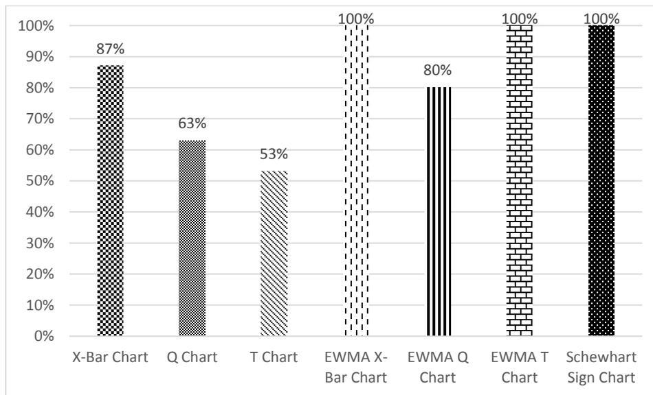
Figure 4.12 Success Rates of the Different Charts to Detect 0.6  $\sigma$  Mean Shift
