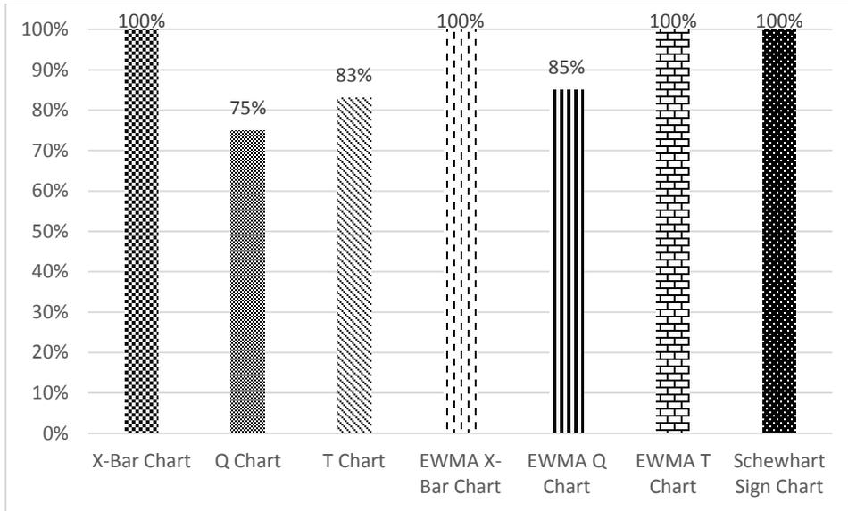
Figure 4.16 Success Rates of the Different Charts to Detect  $1.0 \sigma$  Mean Shift
