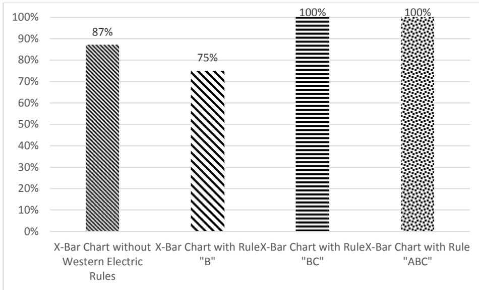
Figure 4.14 Success Rates for  $\bar{x}$  Chart before and after Applying Western Electric Rules
