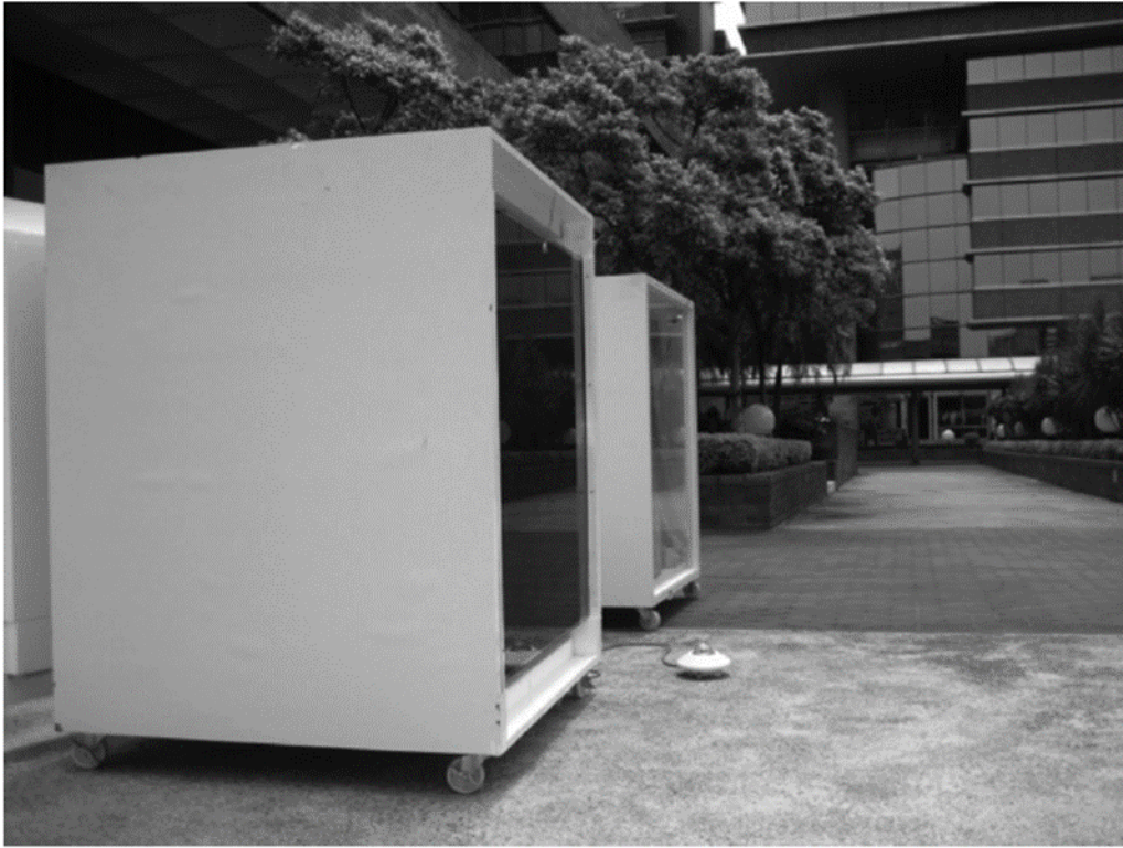
Figure 2.15: Two outdoor test facilities, one with PV façade (left) and one with internal curtain (right) (Han et al., 2013).
