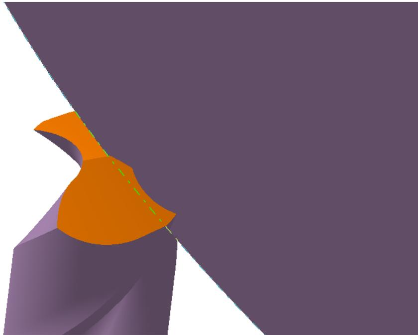
**Figure 3.12 Position and orientation of the grinding wheel for split modeling**
