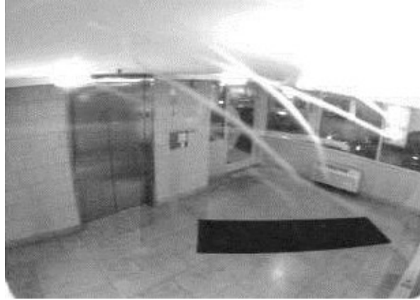
Figure 2-14 Effect of placing the camera behind the lighting source (CheckVideo, 2014)
