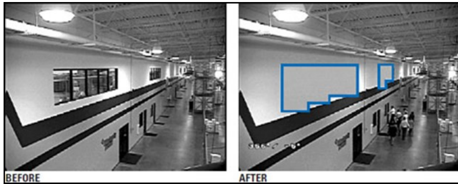
Figure 2-3 Masking feature in PTZ cameras (Kumar, 2012)
