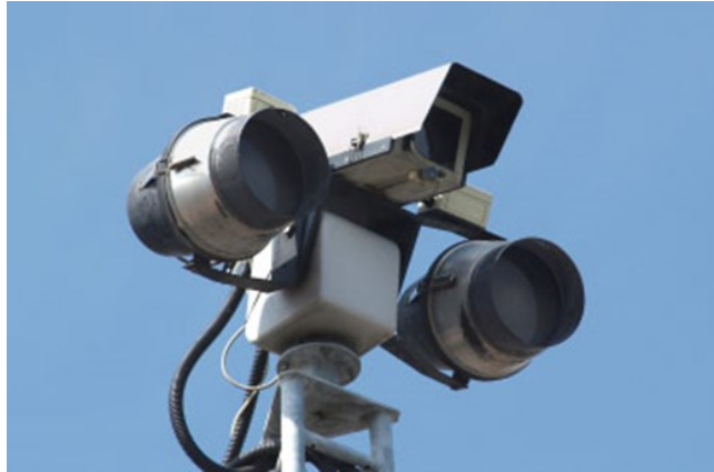
Figure 2-1 Conventional PTZ camera (Kumar, 2012)
