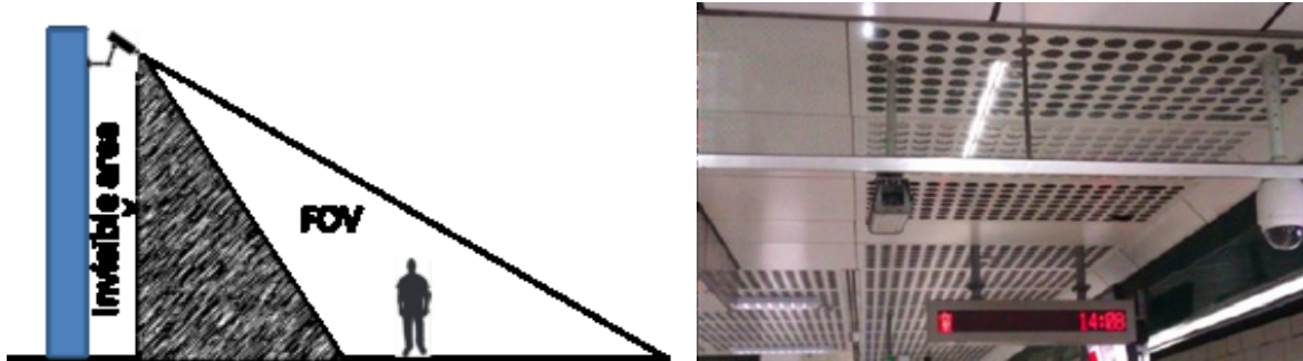
(a) Invisible area under the FOV of the camera
