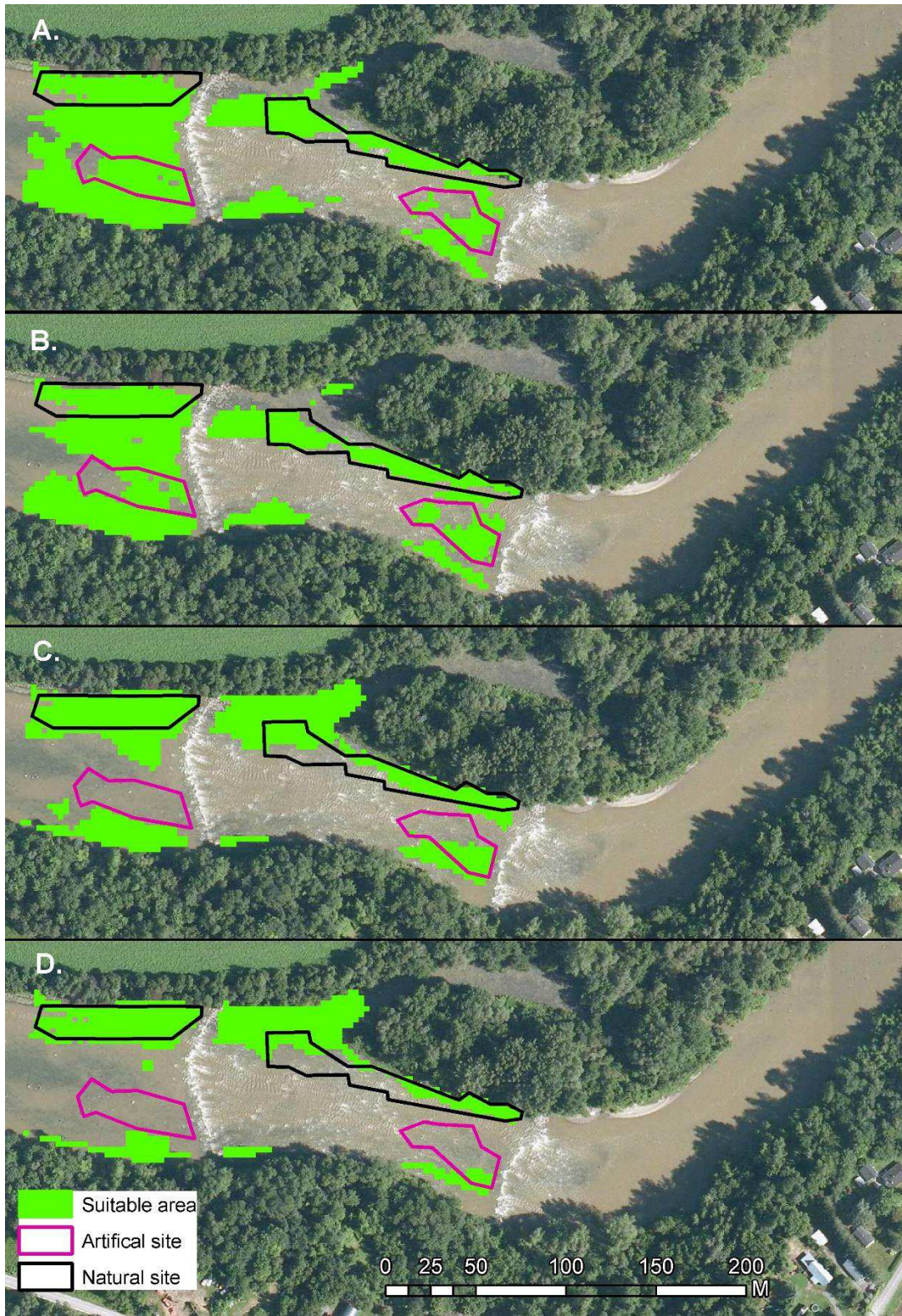
Figure 2.5. Results for the fuzzy habitat suitability model for lake sturgeon spawning at discharges of A. 38 m 3 /s, B. 55 m 3 /s, C. 69 m 3 /s and D. 87 m 3 /s.
