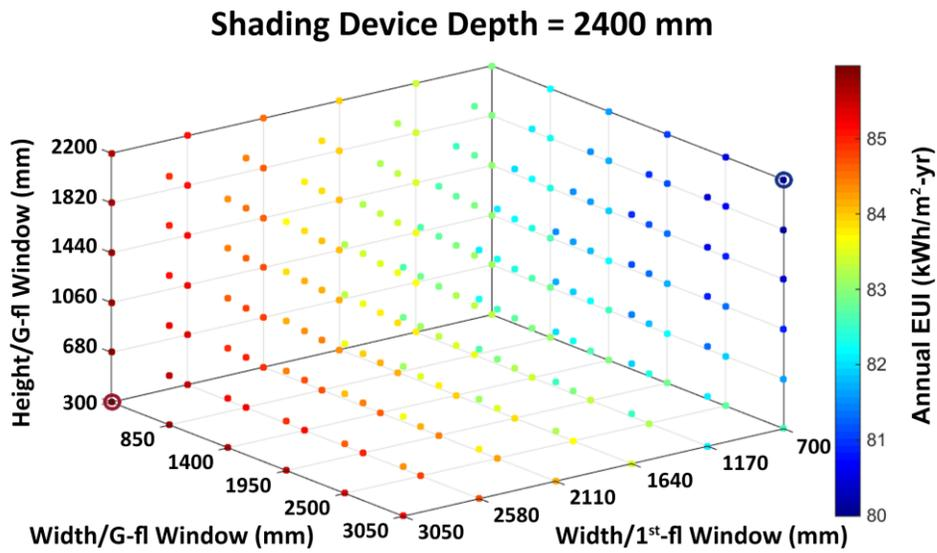
Figure 6.3: Comparison between energy performance of design alternatives due to different depths of the shading device
