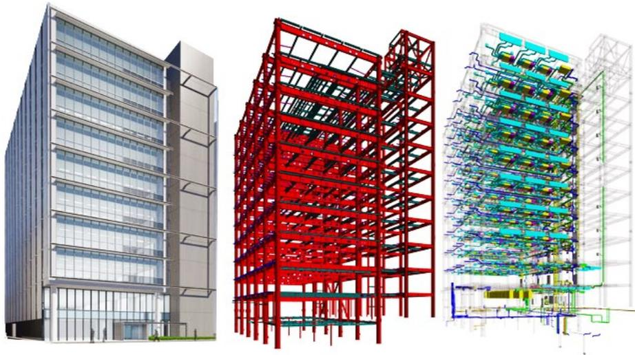
Figure 2.5: i) Architectural ii) Structural iii) MEP models in BIM (AECMAGAZINE, 2011)
