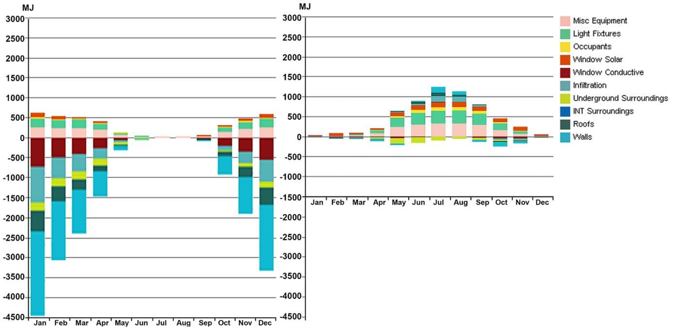
Figure 6.5: Least energy efficient design (no. i), monthly heating & cooling load
