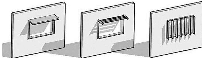
Figure A.4: Common types of exterior overhang and vertical fins, from left to right; overhang, louvered overhang, vertical fins (Robertson and Athienitis., 2009)
