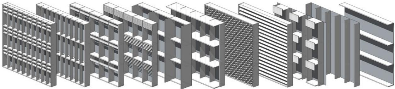
Figure 4.5: Various types of Brise-soleil (Urbanalyse, 2012)
