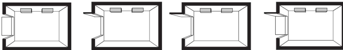
Figure A.5: From left to right; vertical fins, shallow overhang, deep overhang, integrated deep overhang & vertical fins (Carmody and Haglund., 2006)
