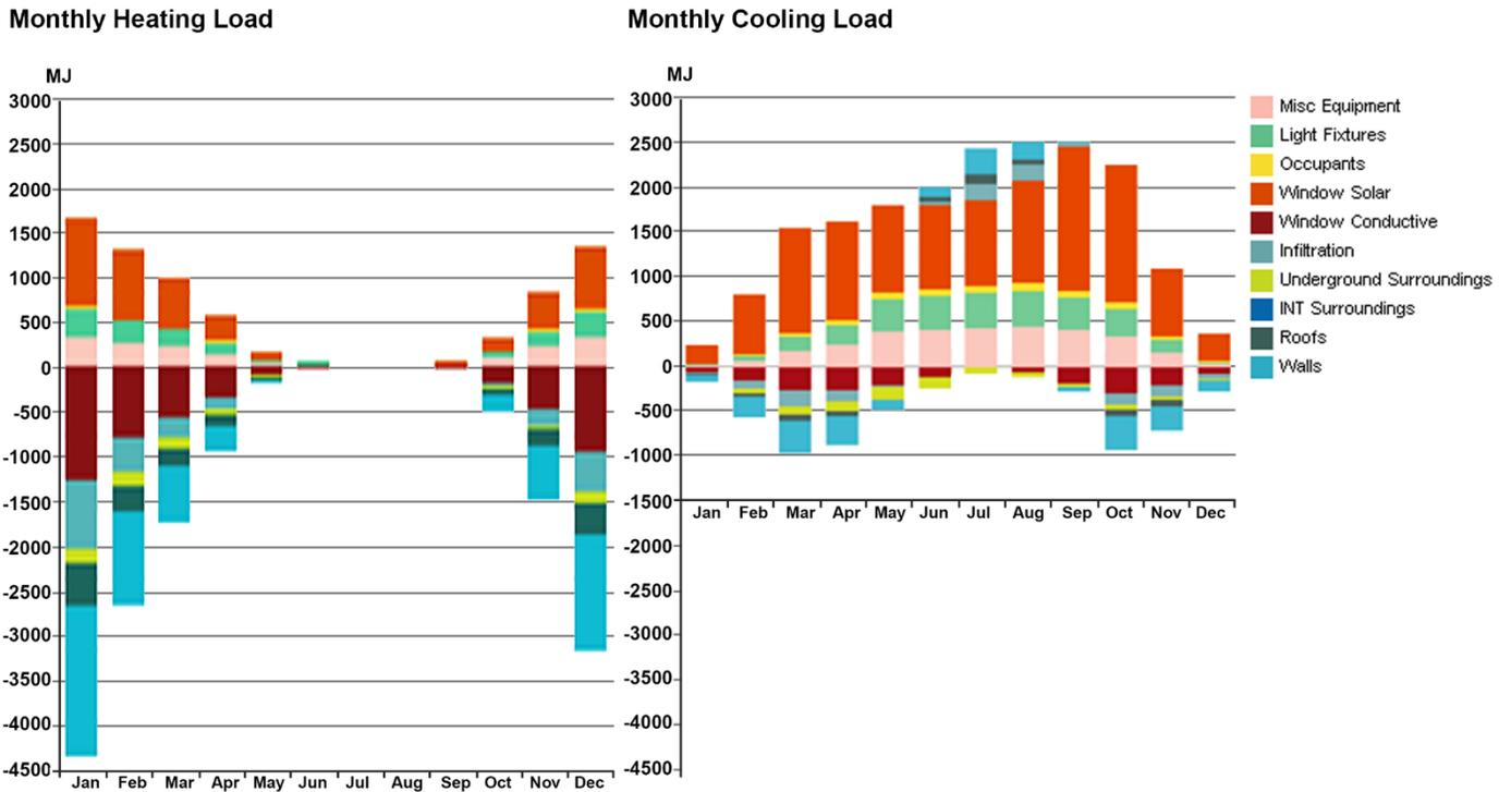
Figure 6.6: Least energy efficient design (no. v), monthly heating & cooling load
