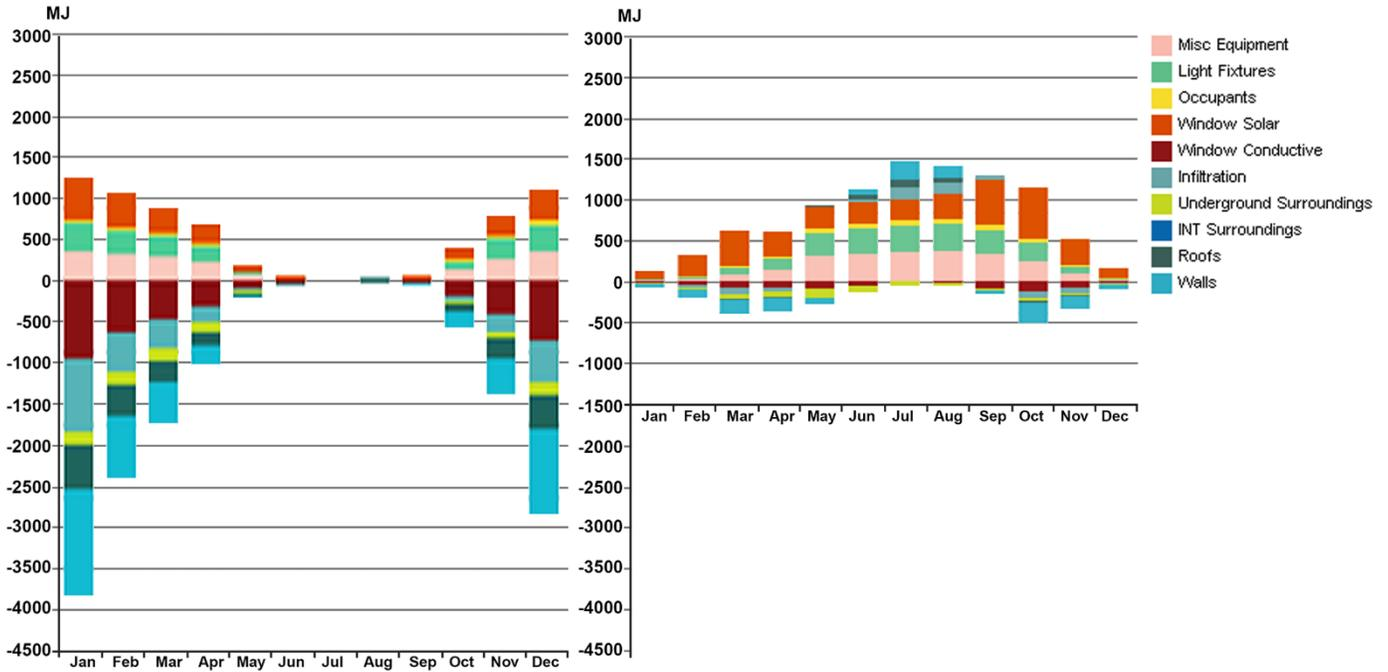
Figure 6.4: Most energy efficient design (no. iii), monthly heating & cooling load
