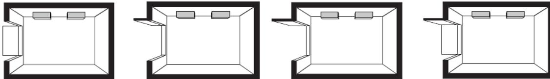
Figure A.5: From left to right; vertical fins, shallow overhang, deep overhang, integrated deep overhang & vertical fins (Carmody and Haglund., 2006)
