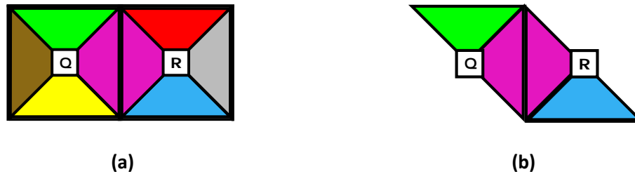
Figure 1.6 A unit DNA computation in the context of EMPs. (a) The alignment of two tiles as a unit action in the process of solving an EMP. (b) The same action conceptually perceived as the alignment of the two relevant half-tiles. (c) The alignment (“stapling”) of two half-tiles by a stapler strand (or the edge-matching “rule”) through strand complementarity. Ligation follows, sealing the 5’/3’ meeting point of the two strands.
