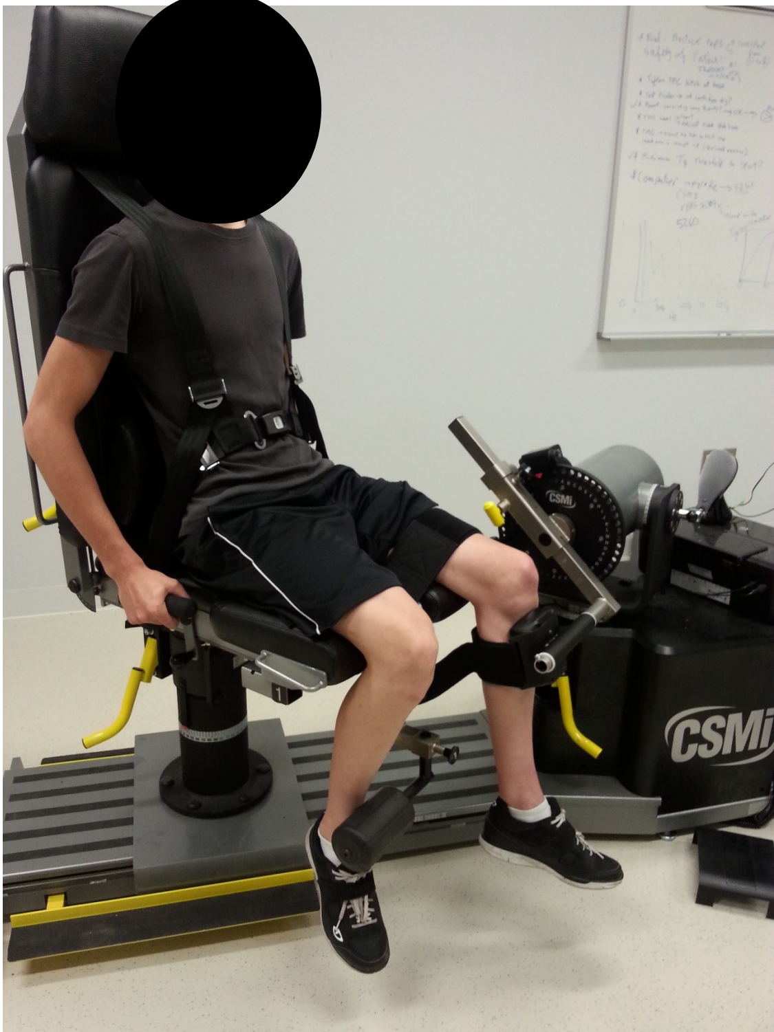
Figure C.1. Humac set-up to test concentric isokinetic knee strength in flexion and extension.
