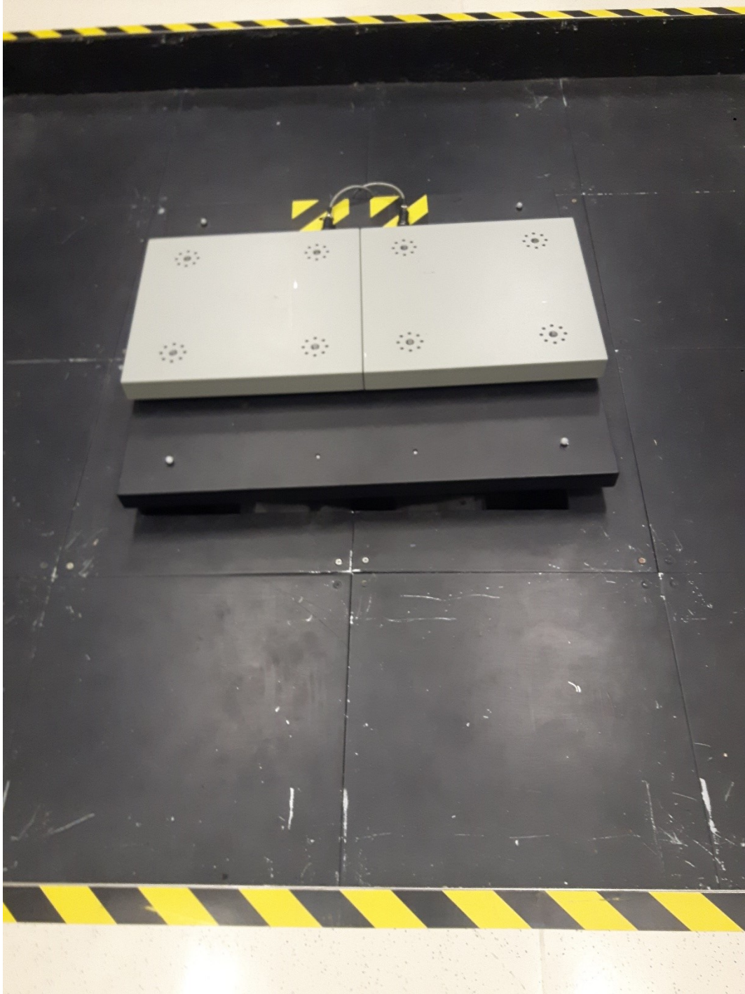
Figure B.2. Custom-made perturbation platform with two force plates mounted on top. Participants stood on one of the force plates during balance testing.
