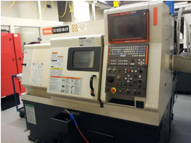
Fig. 4-1. Mazak CNC lathe used for machining of samples.
