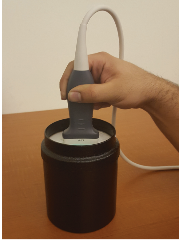
Figure 4.3: Setup for phantom studies: The probe is hand-held during data collection from a CIRS elastography phantom. An excitation with period of 160\mu\text{s} at the focal depth of 20mm is applied as ARF and a set of 80 RF frames were acquired to monitor the shear-wave.
