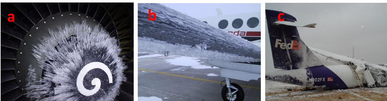
Figure 1-1: Examples of unfavorable and catastrophe of ice accretion, a) Ice accumulation on the spinner of a jet engine [2], b) ice growth on the surface of the airfoil [3], and c) Avionic catastrophe as the result of airframe icing [4].
