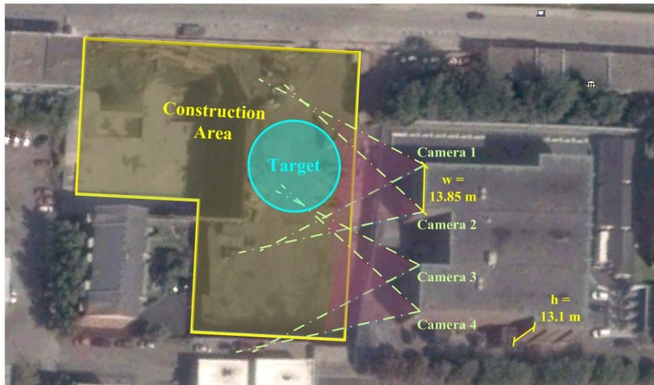
**Figure 5-11. Site layout and cameras' configuration**
