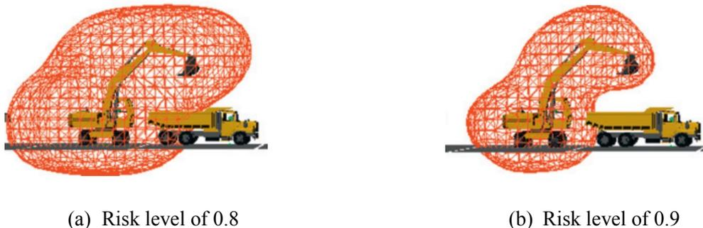
**Figure 2-3. Side views of LAEW of the truck (Vahdatikhaki & Hammad, 2015b)**
