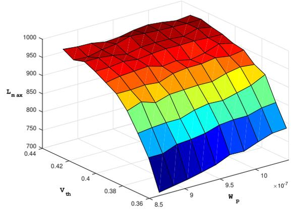
Figure 6.9:  $L_{max}$  variation with the PMOS transistor width and threshold voltage
