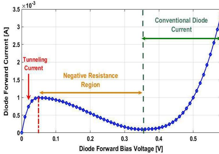
Figure 5.5: Tunnel diode V-I characteristic
