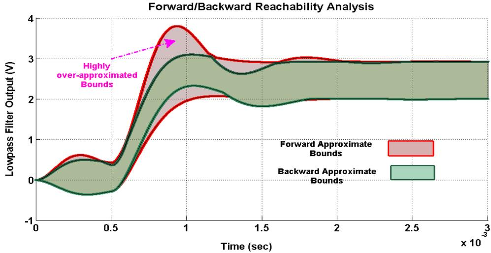
Figure 5.10: Intertwined forward/backward reachability analysis of PLL under jitter
