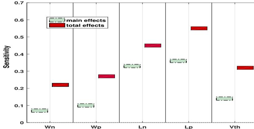
Figure 6.6: Process parameters prioritization for ring oscillator
