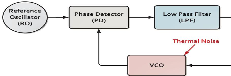
Figure 4.9: Conventional PLL block diagram
