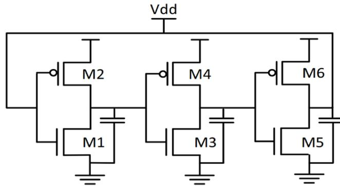
Figure 3.8: Three stage CMOS ring oscillator
