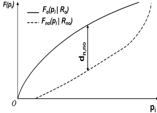
Figure 3.4: Sensitivity index for circuit parameter  $p_i$
