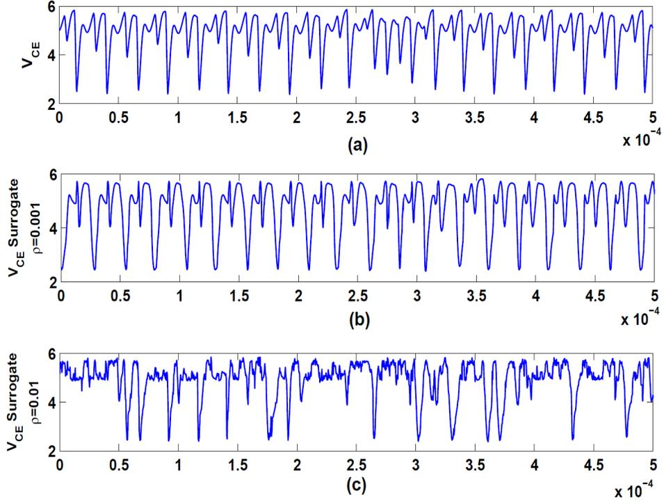
Figure 4.4: The  $V_{CE}$  output and its surrogate for different noise radius  $\rho$
