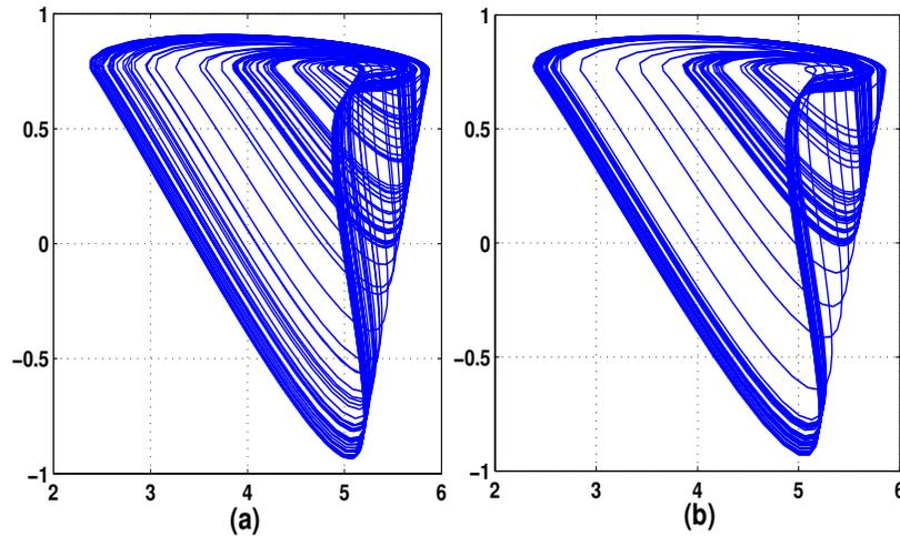
Figure 4.3: Original attractor of Colpitts output (a), reconstructed attractor (b)
