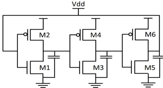
Figure 6.16: Three stage CMOS ring oscillator
