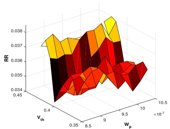
Figure 6.11: Recurrence rate while varying the PMOS transistor width and threshold voltage
