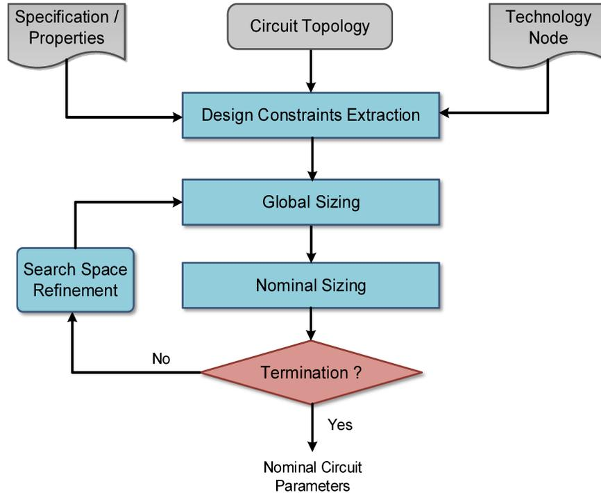
Figure 3.1: Proposed circuit sizing methodology
