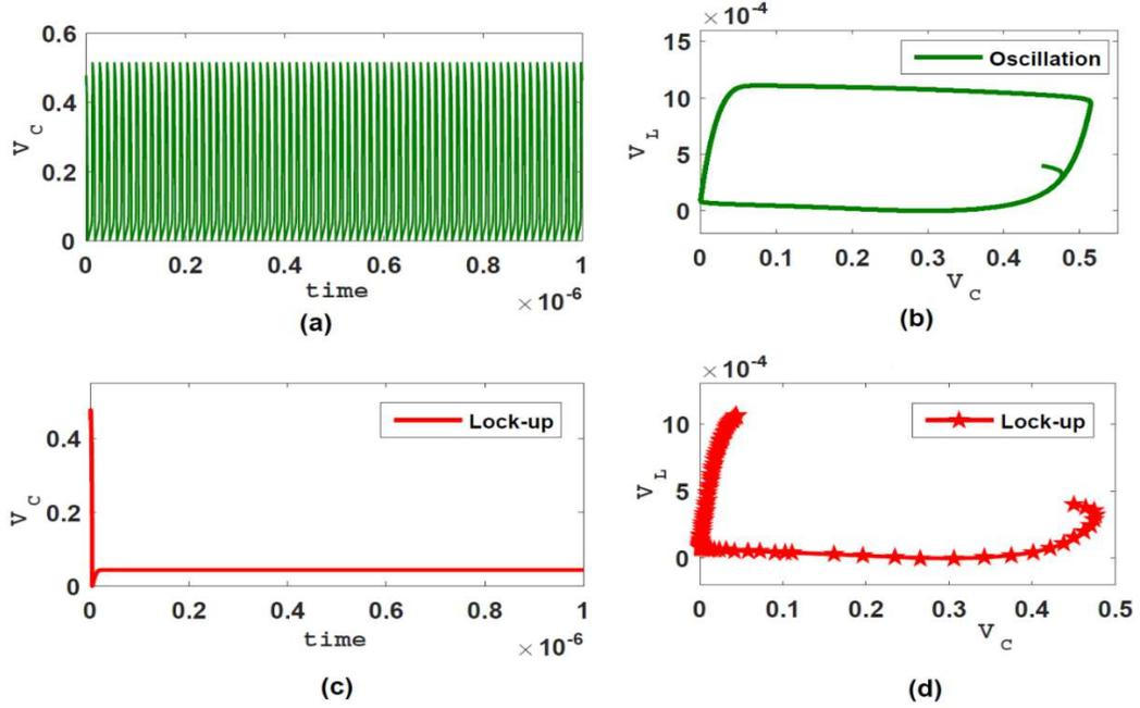
Figure 5.6: Tunnel diode oscillator output for different conductance  $G$
