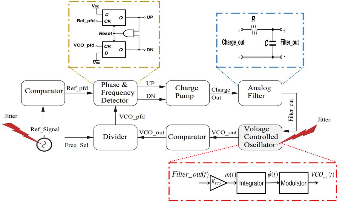
Figure 5.8: PLL design block diagram
