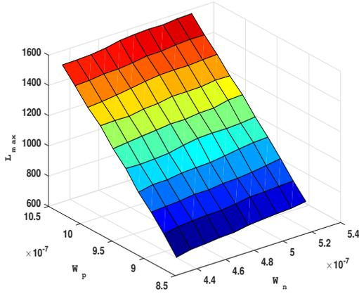
Figure 6.8:  $L_{max}$  variation with the transistors width
