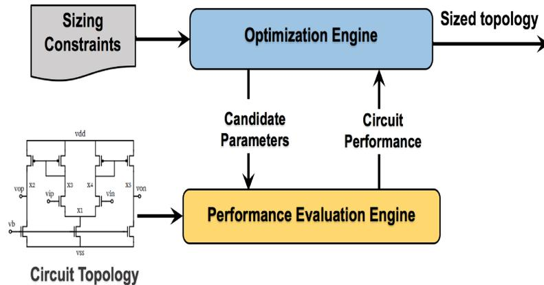
Figure 3.5: Typical analog IC sizing flow
