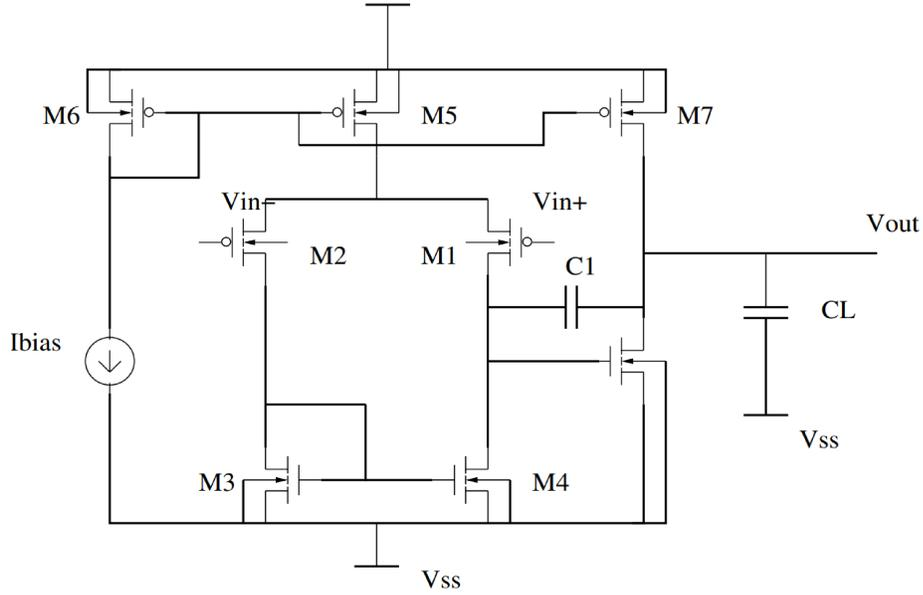
Figure 3.9: Two stage operational amplifier circuit
