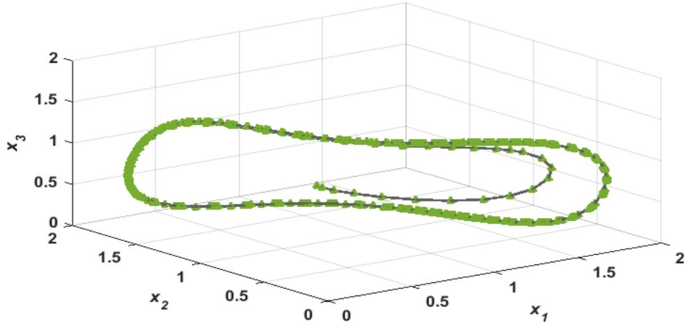
Figure 6.17: Attractor of the optimized ring oscillator circuit
