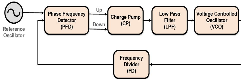
Figure 6.12: Conventional PLL frequency synthesizer
