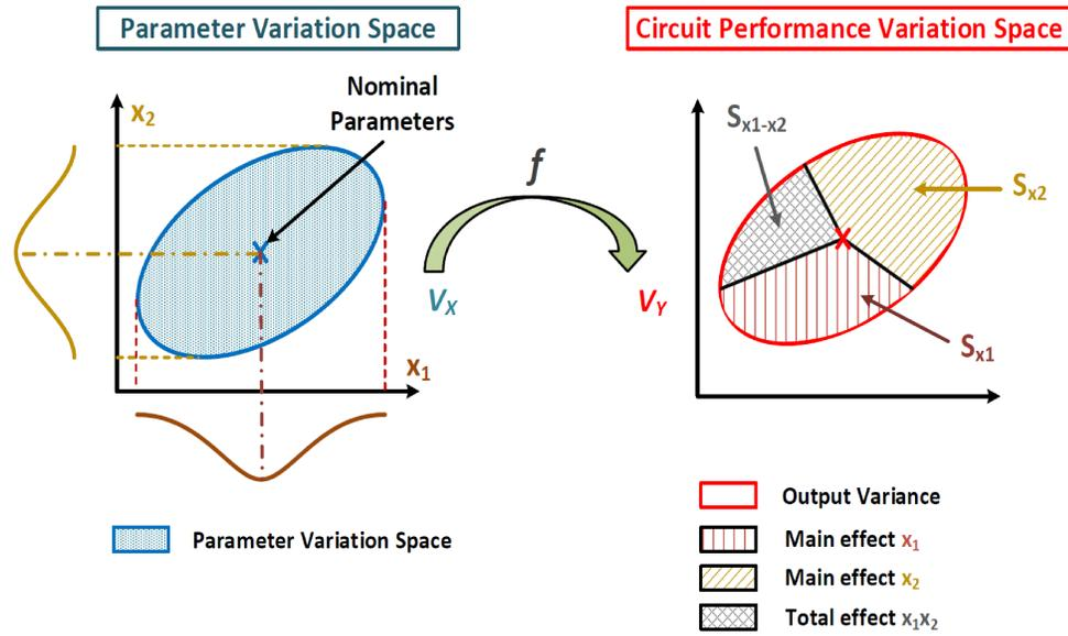
Figure 2.1: Illustration of the global sensitivity analysis concept in a 2-D parameters space
