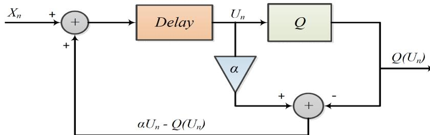
Figure 4.14: First order  $\Sigma$ - $\Delta$  modulator
