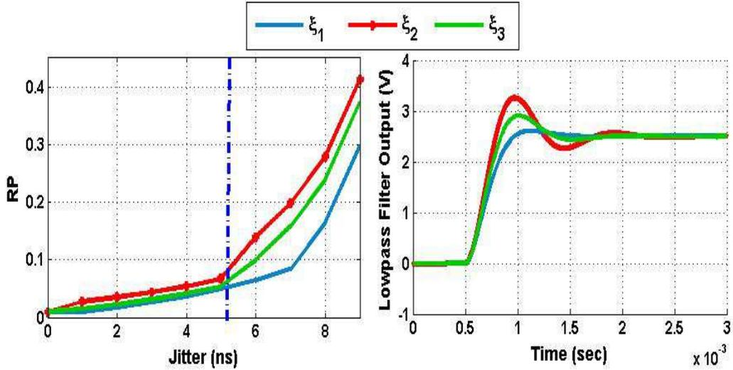
Figure 6.13: Recurrence periodicity for different damping factors
