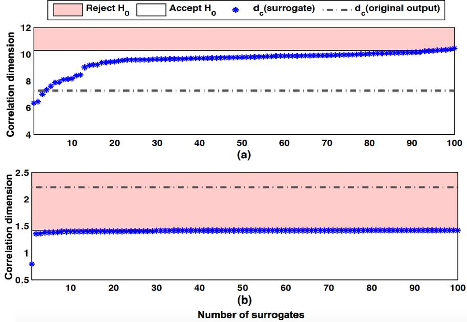
Figure 4.8: Chaos verification for noisy modulator (a), and modulator fed with chaotic input (b)
