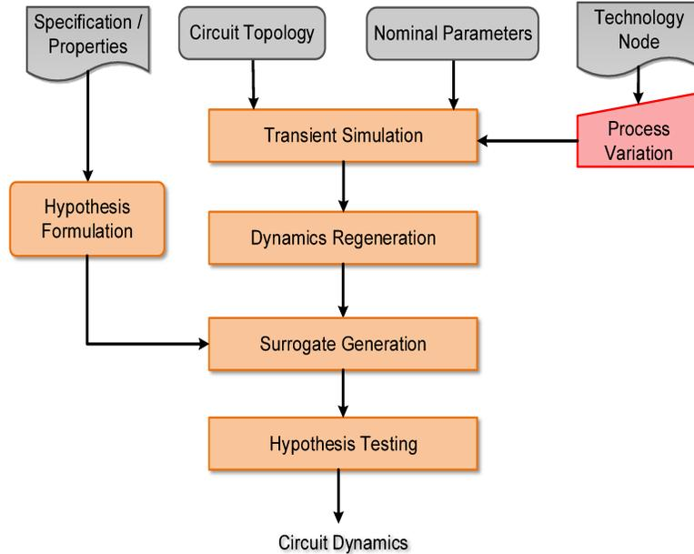
Figure 4.1: Surrogate based chaos/noise verification methodology
