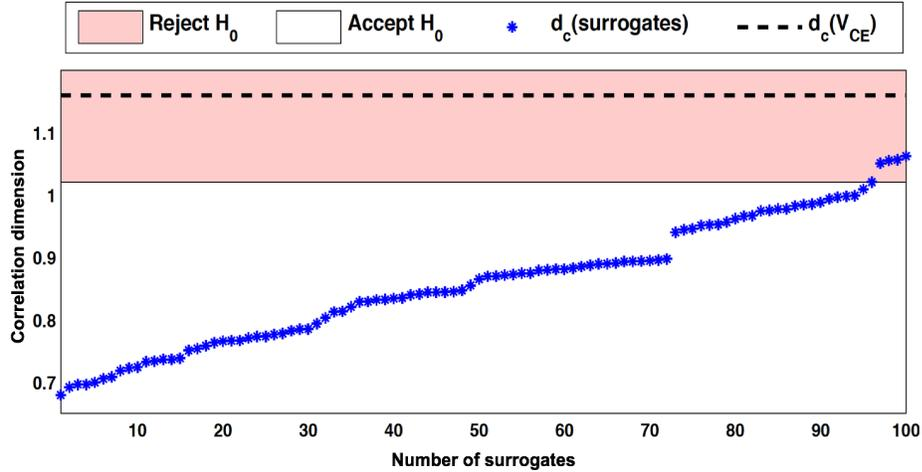
Figure 4.5: Analysis results for chaotic Colpitts circuit
