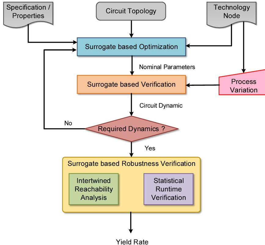
Figure 1.1: Proposed surrogate based optimization and verification methodology
