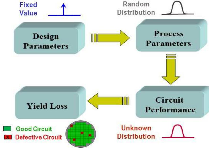
Figure 2.3: Illustration of the process variation effect on circuit yield
