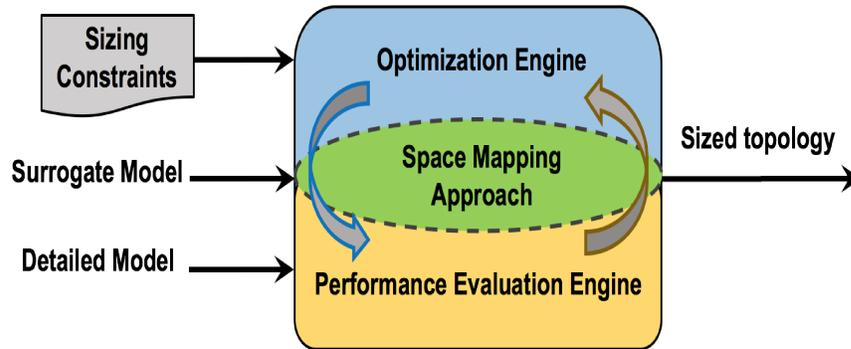
Figure 3.6: Proposed space mapping based nominal sizing flow
