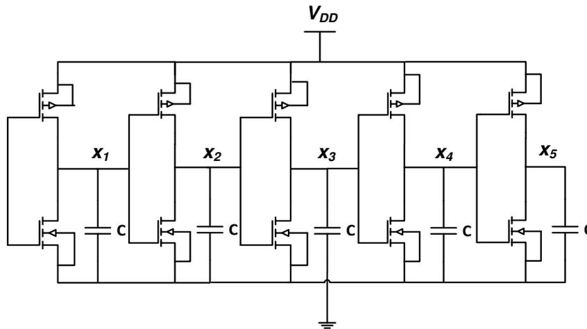
Figure 6.3: Five stage CMOS ring oscillator
