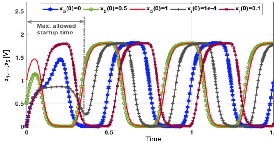
Figure 6.4: Start-up time dependency on the initial conditions
