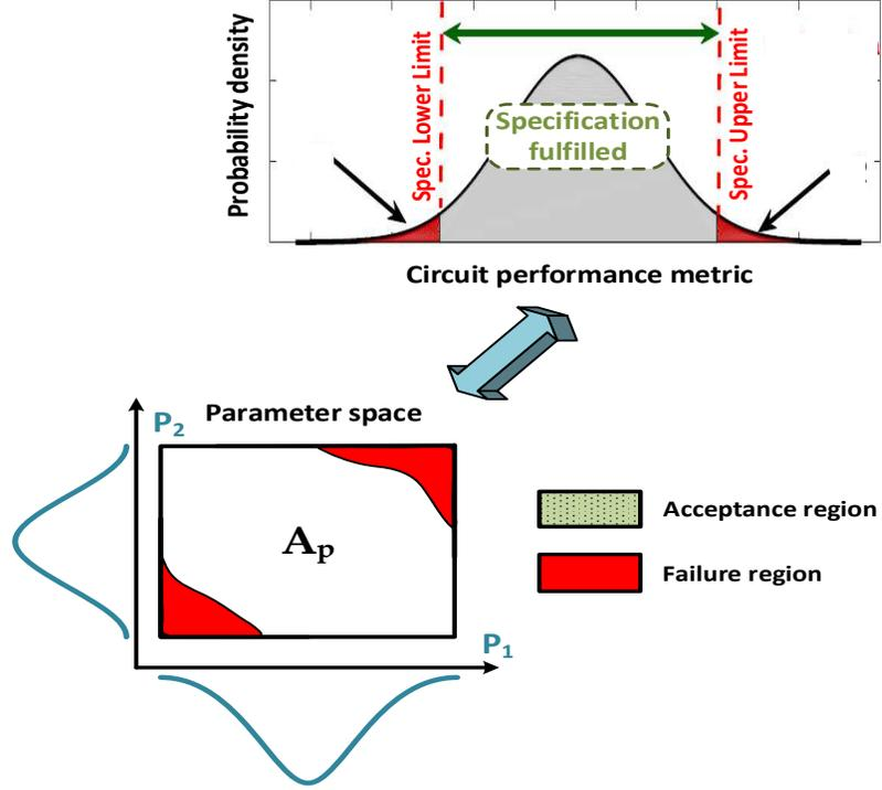
Figure 2.4: Geometrical illustration for 2-D space parameter and a single circuit performance
