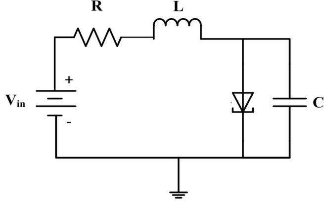
Figure 5.4: Tunnel diode oscillator schematic
