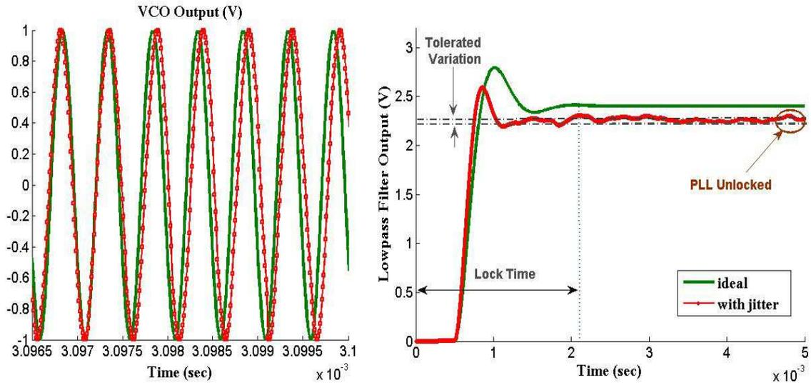
Figure 5.9: PLL output with and without jitter
