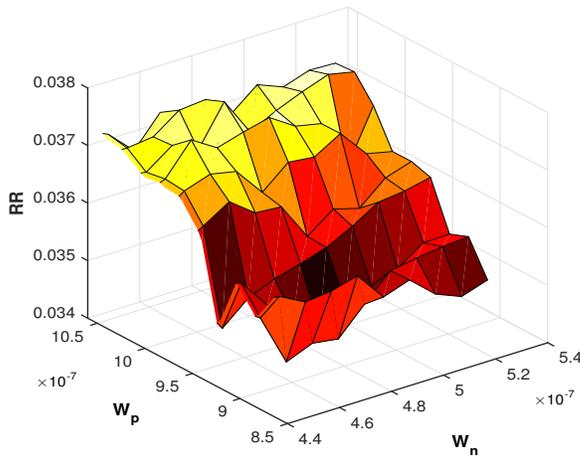
Figure 6.10: Recurrence rate while varying the PMOS and NMOS transistors width
