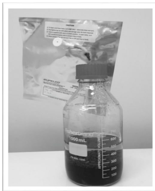
Figure 3.1 1000 mL bottle with septum cap and gas collection bag used for batch tests.
