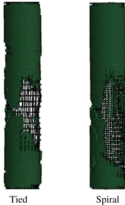
Figure 6.7 Side view of the Vancouver spiral columns at the end of simulations, Case I, X2.
