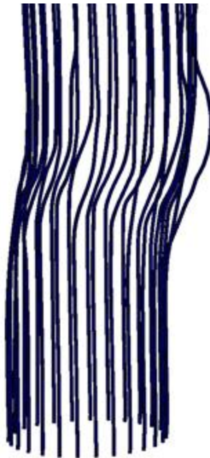
Figure 5.15 Deformation of longitudinal bars for the Toronto tied column, Case II, X1.
