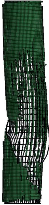
Figure 6.2 Erosion at the base of the Toronto tied column at 38 ms, Case I, X2.
