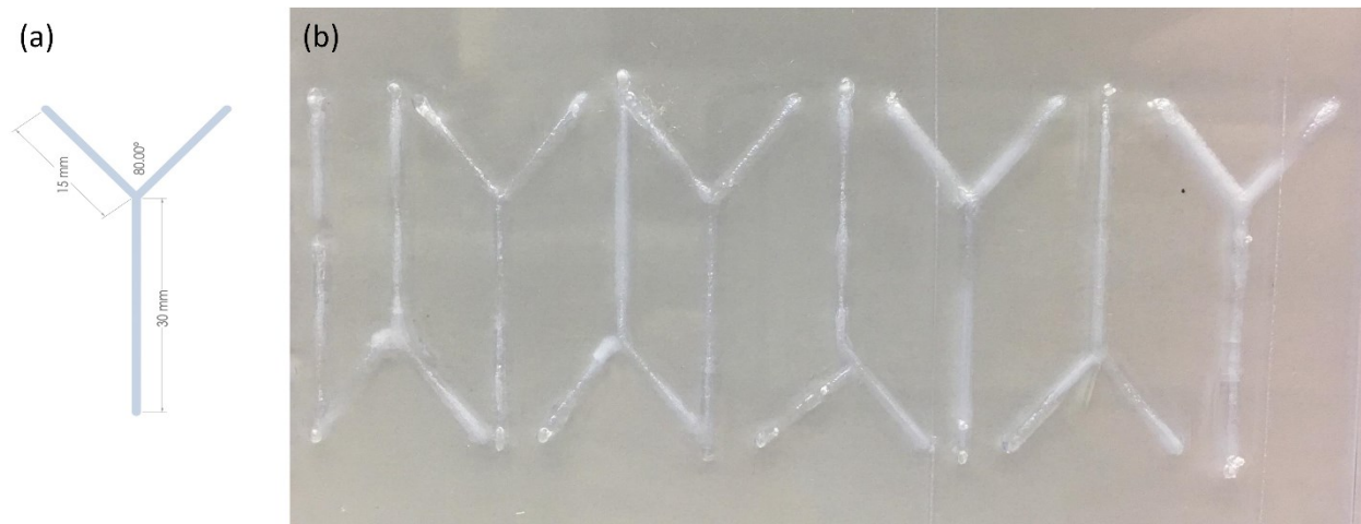
Figure 7-10 Mold fabrication by a HIFU transducer. (a) designed model (b) Fabricated acrylic molds at a duty cycle of 60 % and with various feed rates; the second model from the left was chosen for mold fabrication.
