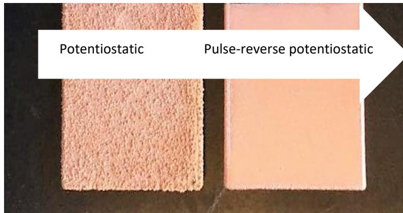
*Figure 3-27. Copper deposits made by potentiostatic plating and pulse-potentiostatic plating modes from left to right, for the same charge of  $10 \text{ C/mm}^2$*
