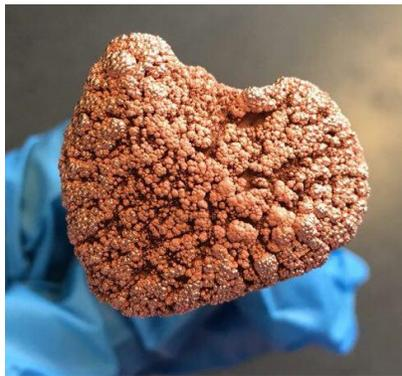
*Figure 3-34. Copper electroformed plaster part (potentiostatic mode, - 0.3V applied potential).*
