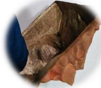
*Figure 3-31. Copper electroforming of a non-conductive 3D printed ABS part **Above)** Right to left: Galvanostatic copper electroformed part, potentiostatic copper electroformed part, pulse-potentiostatic copper electroformed part **Below)** View from inside the hollow part*
