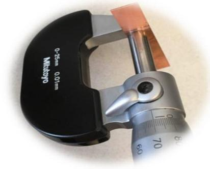
*Figure 2-8. Coating thickness measurement using a micrometer*
