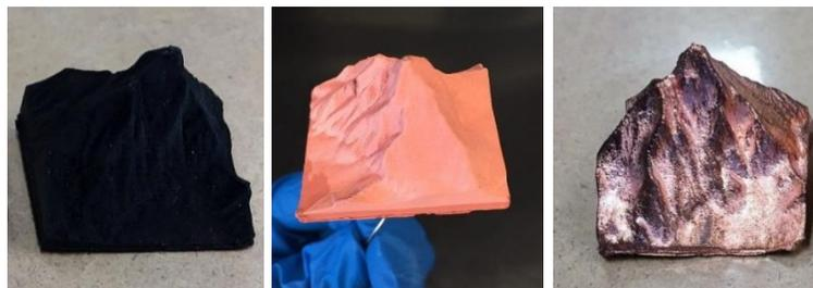
*Figure 2-11. Left: ABS printed part, Middle: Electroless copper plated ABS part, Right: Copper electroforming of electroless copper plated part*
