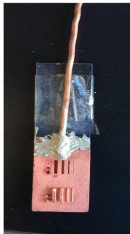
*Figure 3-37. Copper electroforming of a SLA printed part (electronic chips)*
