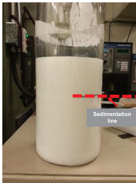
Fig. 20. Sedimentation line marked on the container of suspension used in the spray process of SPS-W-0 at the end of the SPS process.
