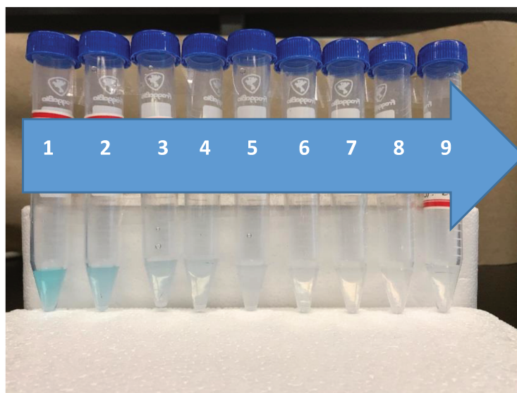
Fig. 51. Degradation of methylene blue by decoloration of the solution in the presence of SPS \text{TiO}_2 membrane.
