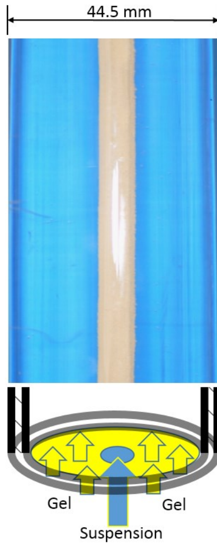
Figure 2-10 Steady flow of Titania 50 wt. % lubricated by Carbomer 0.2% gel, Q_{\text{core}}=5.2 \text{ mL/s} and Q_{\text{lub}}=4.3 \text{ mL/s}
