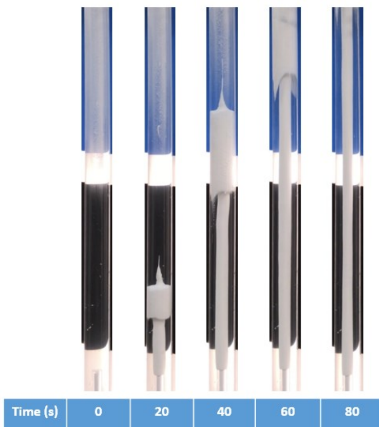
Figure 2-8 Snapshots of the flow of the Titania suspension (white color) and the Carbomer gel
