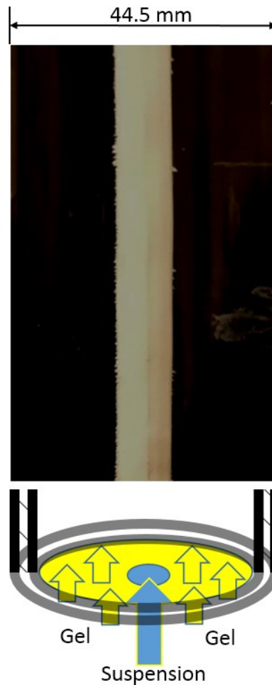
Figure 2-9 Steady flow of Titania 30 wt. % lubricated by Carbomer 0.2% gel, Q_{\text{core}}=7.7 \text{ mL/s}
