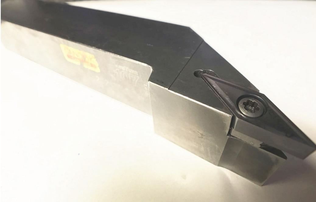
Figure 2.5 A picture of a Korloy VBMT160408 insert and a Sandvik SVJBL 2525M16 tool holder
