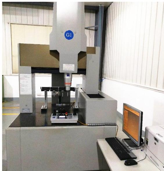
**Figure 2.17 Trilinear coordinates measuring instrument**
