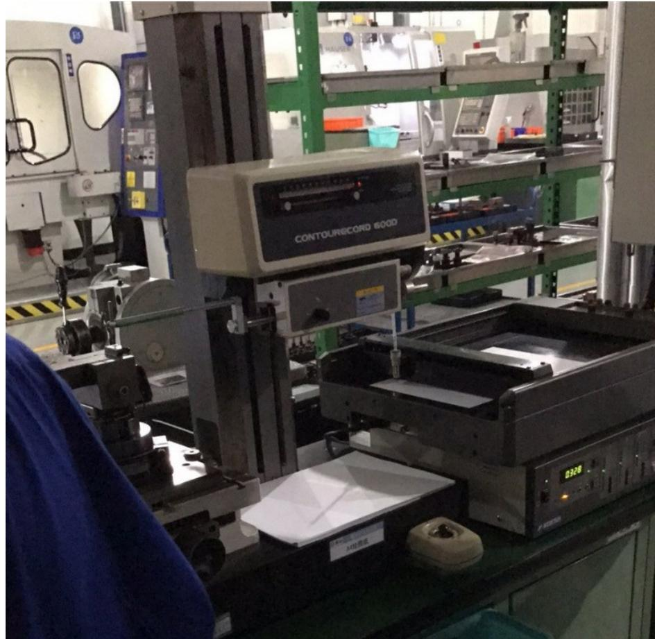
**Figure 2.6** The Korloy® VBMT160408 insert is measured on an electric surface profiler
