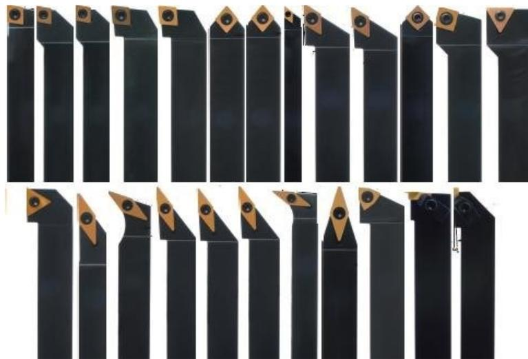
Figure 2.15 A picture of different indexable insert holders
