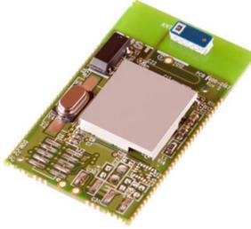
Figure 15: DUST module to mount on the prototype board
