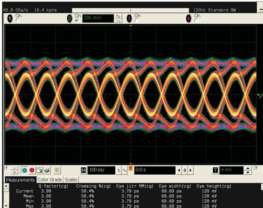
Figure 60: Real-time eye-diagram - 100 ps
