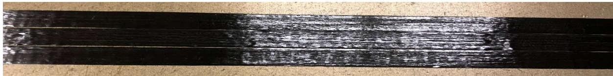
Figure 6.18 Straight path (case 2; speed 50 mm/s, force 133.4 N, temperature 150 °C).
