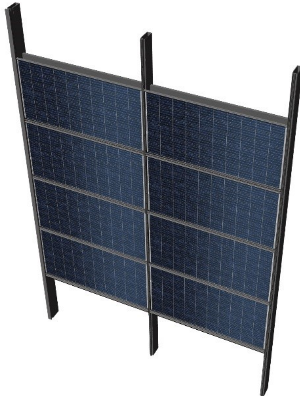
Figure 3.30: Multiple-inlet CW BIPV/T system
