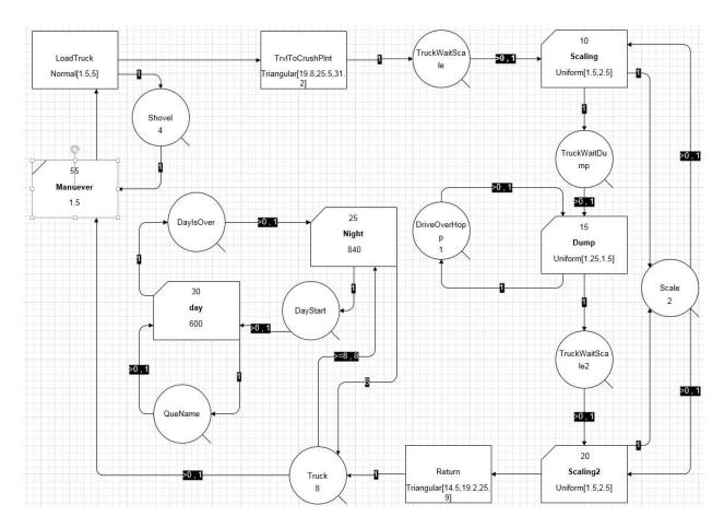
Figure 16. Petri net of the example- an earth moving operation (modeled by EZstrobe stencil )
