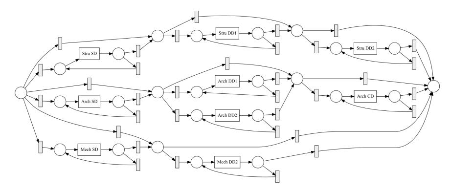
Figure 37. Level 2 BIM process map (as-happened) for design authoring which is illustrated in Petri net format - Case study #2
