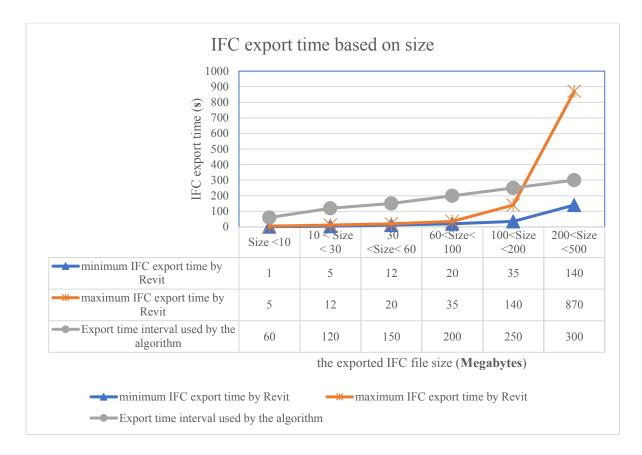
**Figure 7**. IFC export time using Revit 2018 based on the file size (The computer which was used in this project had an Intel(R) Xeon(R) CPU (E3-1270 v5 @ 3.60 GHz) and a 16 GB of RAM.)
