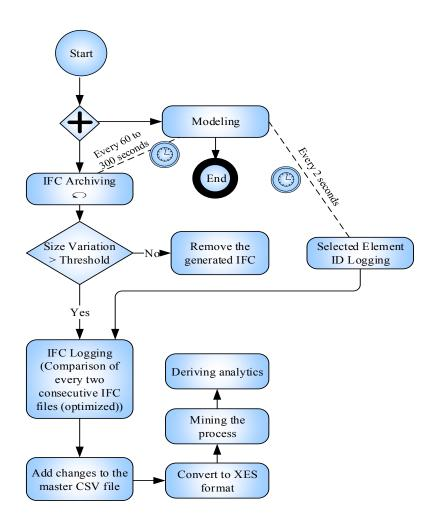
**Figure 6.** BIM – Process Mining integration model: second generation activity diagram (for the second case study)
