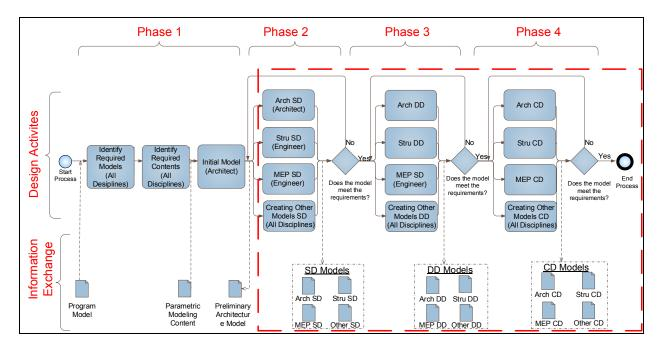
Figure 4. The scope of the methodology: based on level 2 BIM process map [4]
