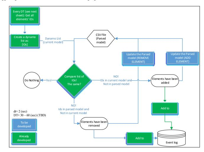
Revit based logger algorithms are illustrated in the following figures:
