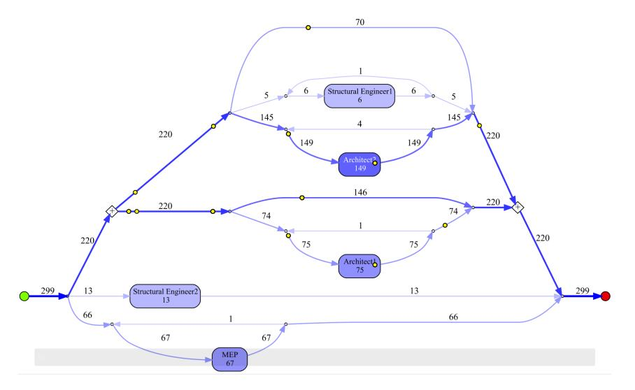
**Figure 25.** level 2 process animation: the number in each box shows the frequency of changes for the elements which are passing through each box (activity) within the project timeline - Case study #1
