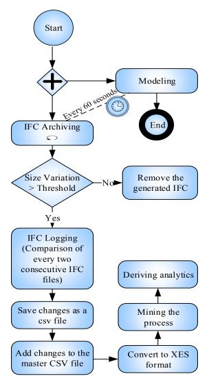
**Figure 5.** BIM – Process Mining integration model: first-generation activity diagram (for the first case study) [2]
