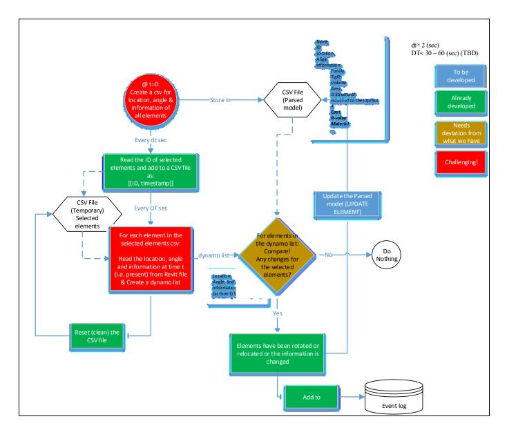
Figure 47. Revit based logger algorithm (rotation, relocation and information changes)
