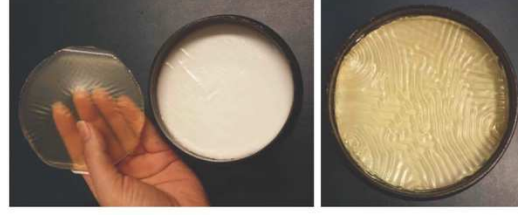
Fig. 2. CIRS phantom and the acoustic gel pad.
