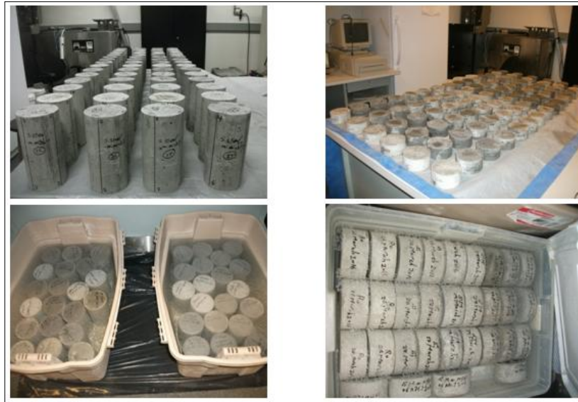
Figure (5.1) Part of fibre reinforcement concrete (FRC) specimens of a different size after de-molding and during curing
