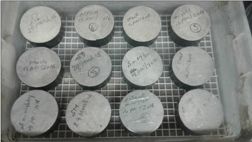
Figure (3.19) Samples preparation before starting sorptivity test
