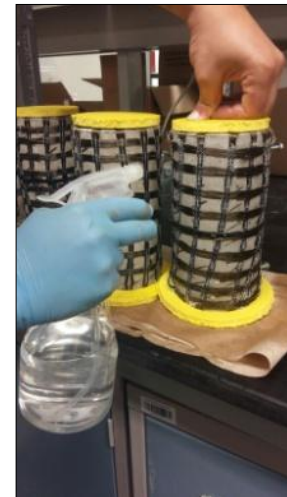
Figure (6.4) Application of lithium nitrate on the specimens surface using topical application
