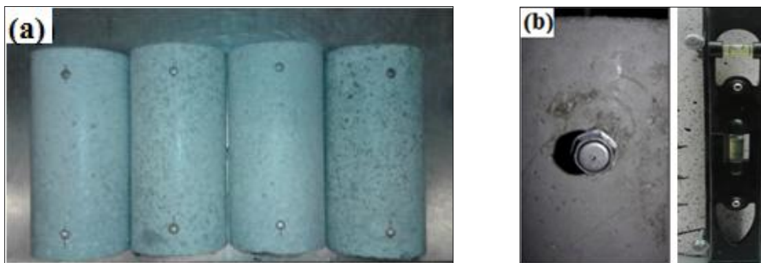
Figure (6.1) Demec installation
