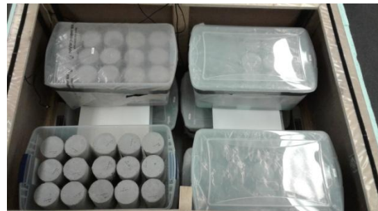
Figure (4.9) Storage of concrete specimens in the environmental room at 38 °C and 95±5% RH
