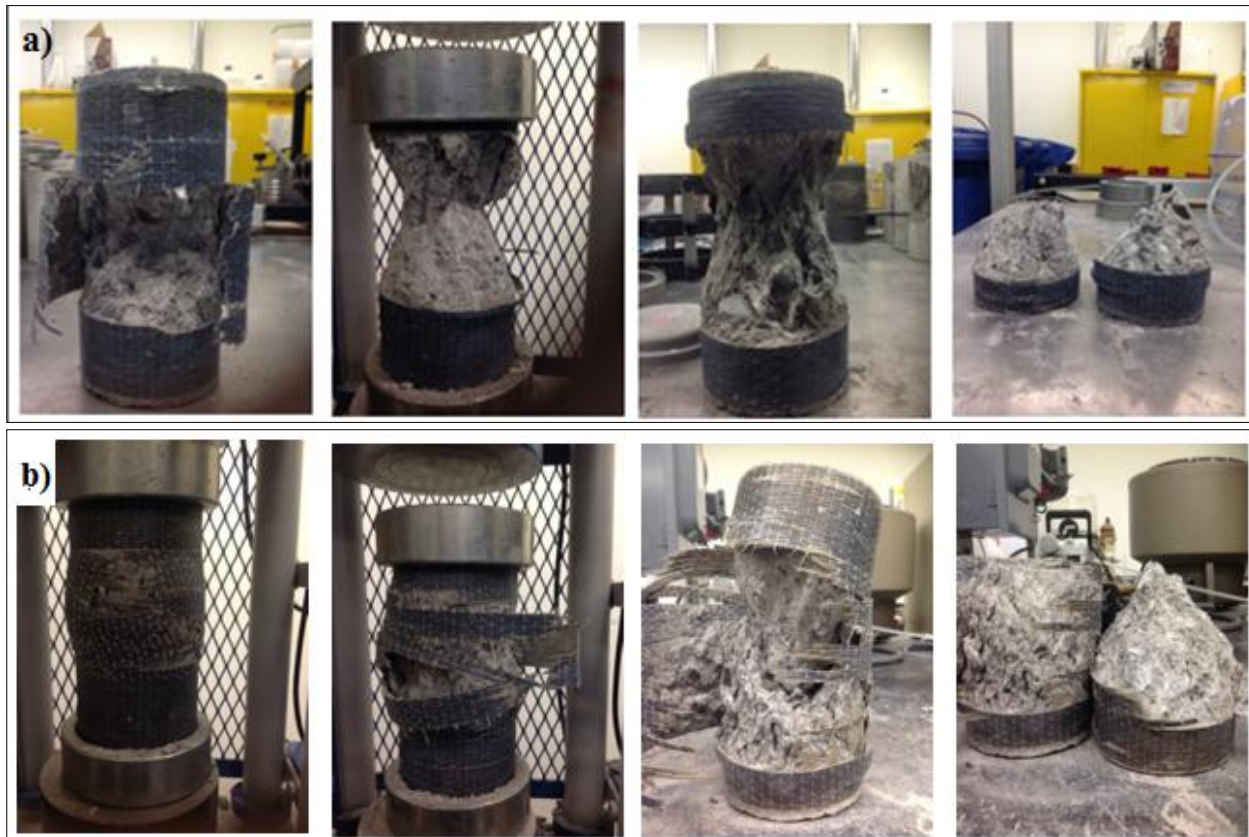
Figure (6.18) Specimens strengthened at 1, 2, 3, and 4 months and tested after 2 months from the strengthening date
