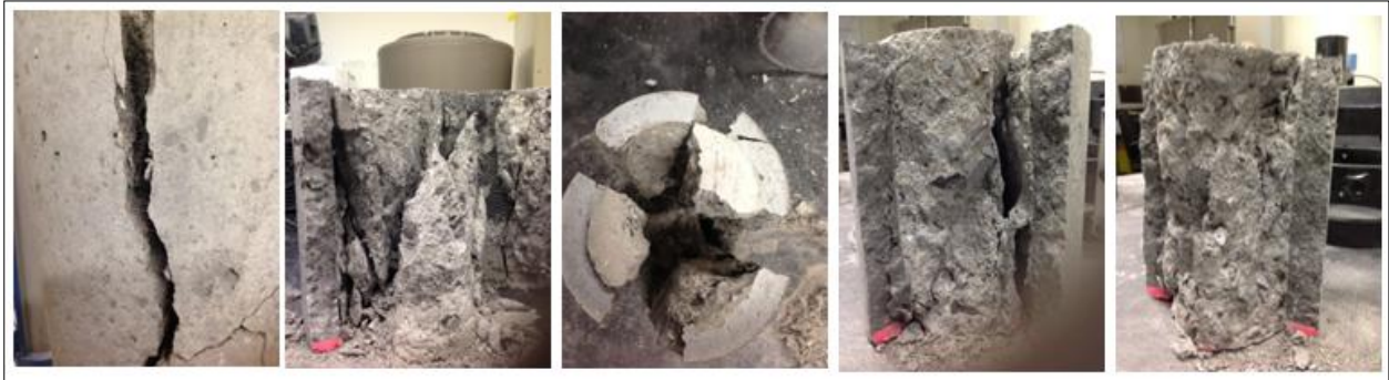
Figure (6.21) Specimens strengthened with FRC jacketing at 1, 2, 3, 4, and 5 months and tested after 4 months from the strengthening date
