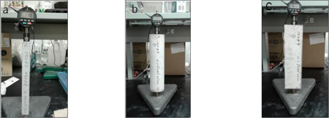
Figure (3.14) Expansion measurements by using digital comparator of accuracy 0.002mm (a) Mortar bar, (b) Concrete prism, and (c) Concrete cylinders
