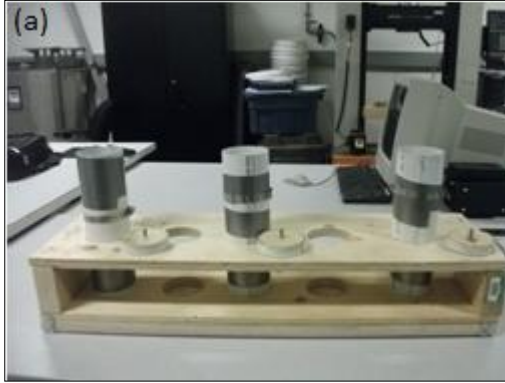
Figure (4.7) Preparation of concrete cylinder specimens (Ø75mm×285mm) (a) Mold of cylinders Ø75mm×285mm, and (b) Mold after casting concrete
