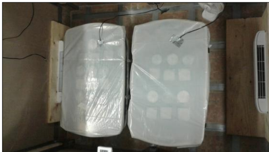
Figure (4.9) Storage of concrete specimens in the environmental room at 38 °C and 95±5% RH
