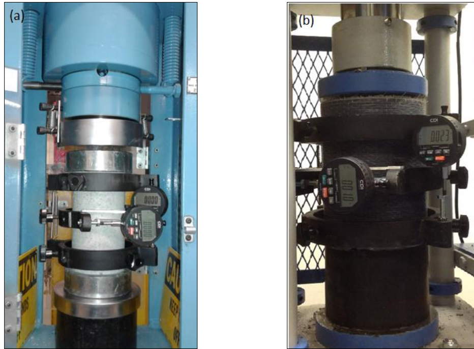
Figure (3.8) Setup of stiffness damage test (SDT) of (a) SDT on Ø100mm×200mm specimens prior strengthening, and (b) SDT after strengthening
