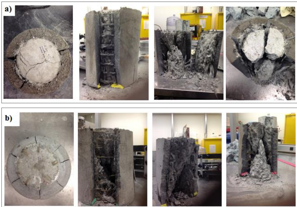
Figure (6.20) Specimens strengthened at 1, 2, 3, and 4 months and tested after 2 months from the strengthening date
