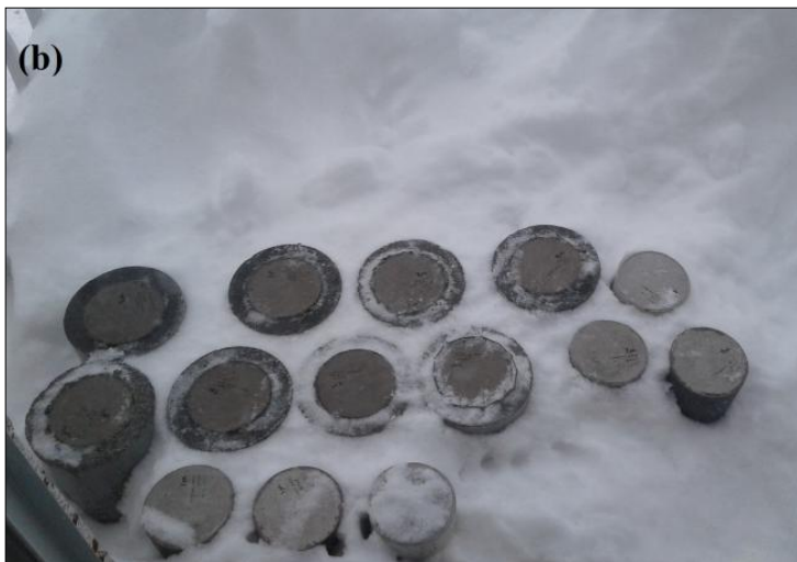
Figure (7.1) Long term exposure condition (a) At 38 °C % 95±5% RH, (b) Actual weathering conditions,
