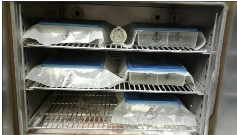
Figure (4.5) Storage of mortar bars in an oven at 80 °C
