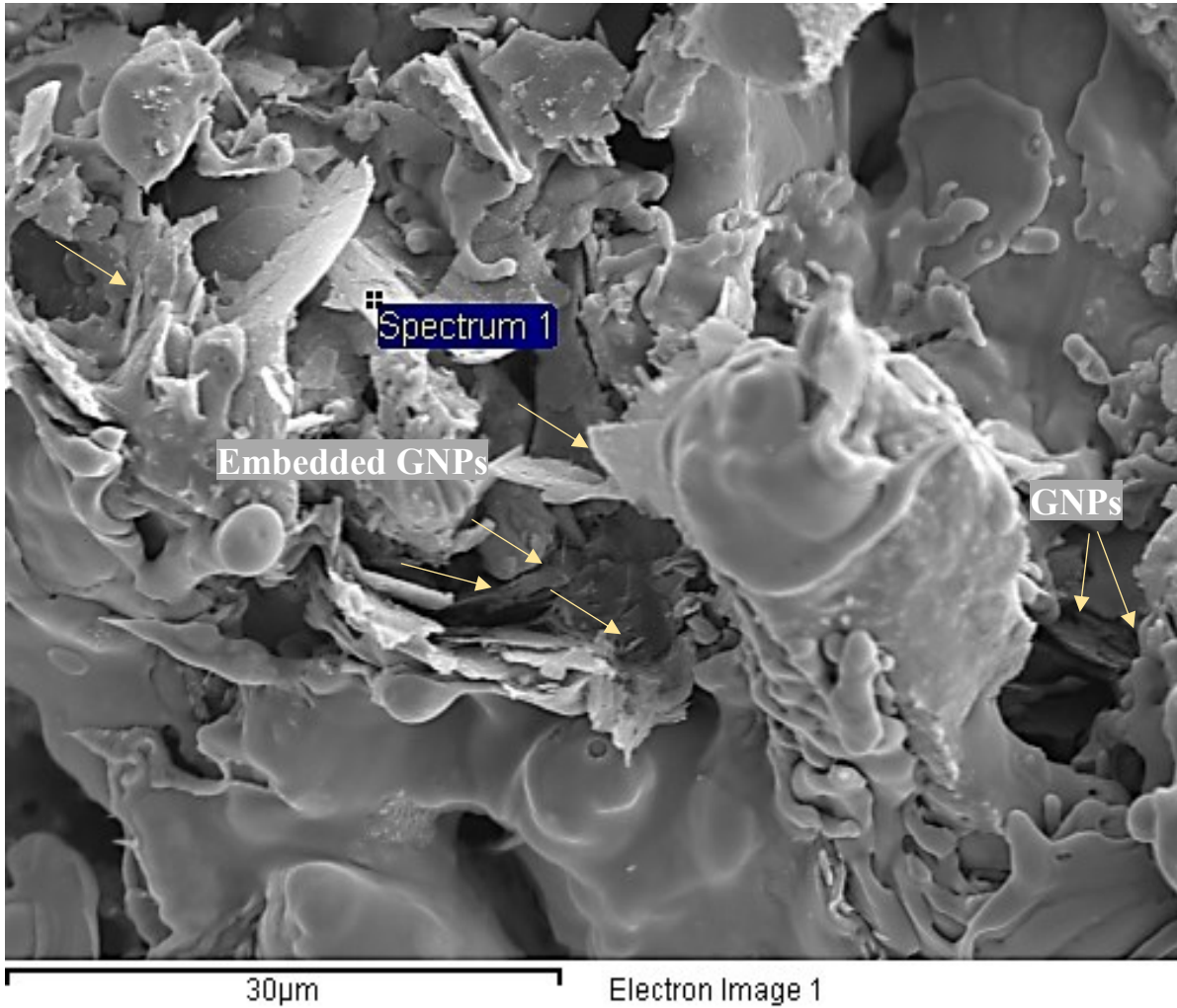
Figure 4-7. SEM Image and elemental mapping of the Cu-GNP-MP-APS-S sample
