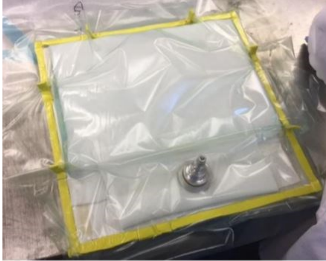
Figure 3-1 schematic of the vacuumed sample before curing
