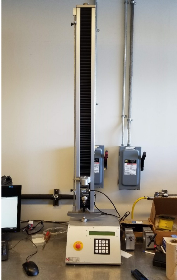
Figure 3-10 Z5 single column tensile tester machine and Wyoming three point bending fixture
