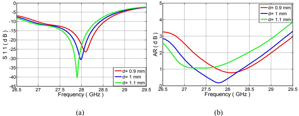
Figure 6.8: Simulated return loss (a) and axial ratio (b) of the proposed CP SIW cavity antenna considering the effect of varying the distance between the antenna and converter [71].
