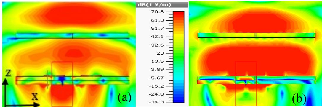
Figure 3.10: Magnitude of the E-field distribution of DD patch antenna array with a conventional superstrate (a) and with a holey superstrate (b) at 28 GHz [93].
