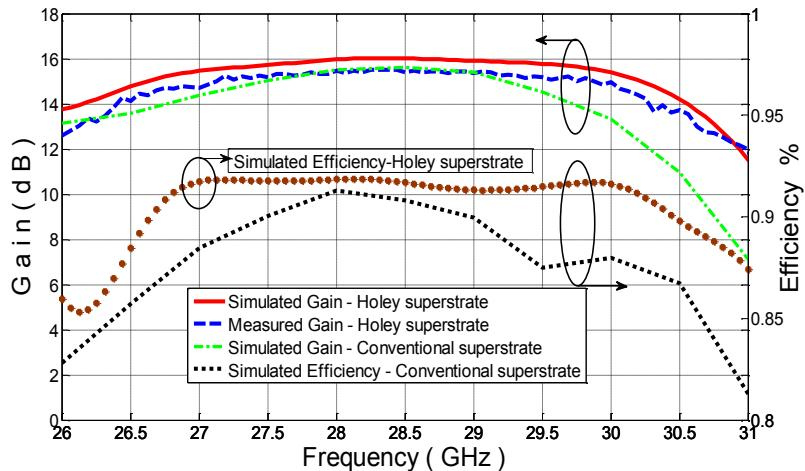
Figure 3.9: Simulated and measured gain and simulated radiation efficiency of the implemented antenna compared to the DD patch array with a conventional superstrate [93].
