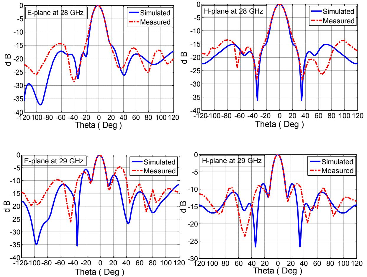
Figure 5.6: E- and H-plane radiation patterns of the proposed antenna at 28 GHz and 29 GHz [91].
