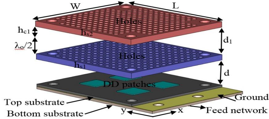
Figure 3.16: Geometry of the proposed antenna: side view.
