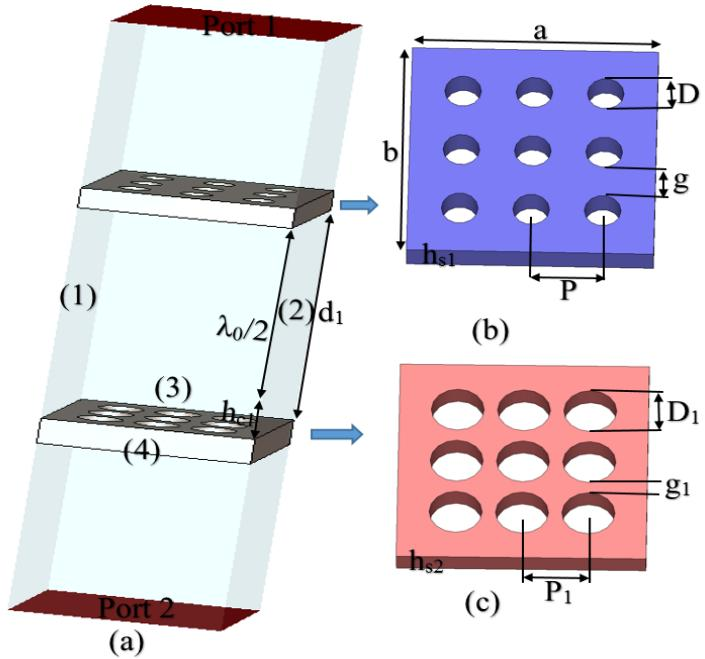
Figure 3.12: Geometry of the proposed unit cell: Characterization model of the unit cell (a), top substrate (b), and bottom substrate (c).
