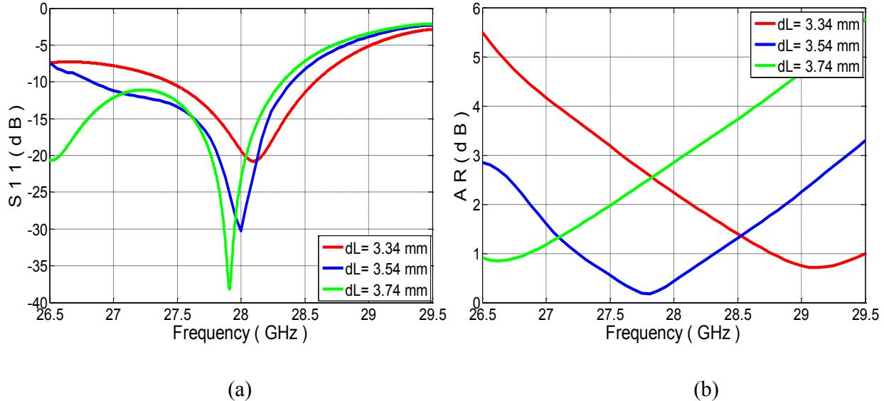
Figure 6.9: Simulated return loss (a) and axial ratio (b) of the proposed CP SIW cavity antenna considering the effect of varying the dipole length [71].
