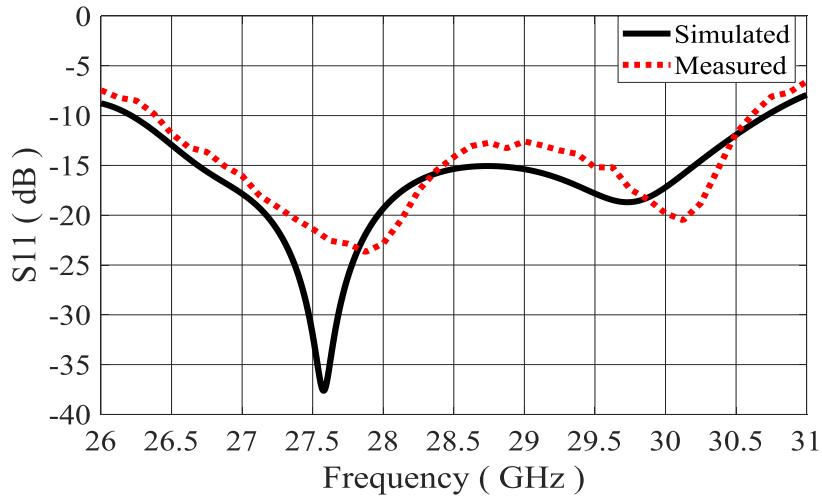
Figure 4.4: Simulated and measured reflection coefficient of the proposed antenna.
