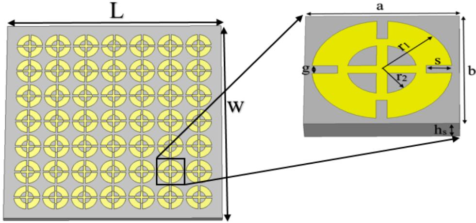
Figure 5.2: Bottom side of the FSS superstrate, and the geometry of the proposed unit cell [91].
