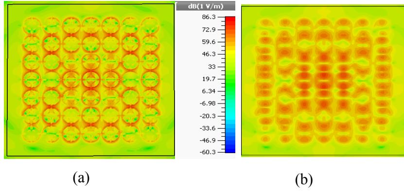
Figure 5.14: E-field distribution of the DD patch antenna with a positive phase at 28 GHz: Bottom of the superstrate (a), and top of the superstrate (b) [91].
