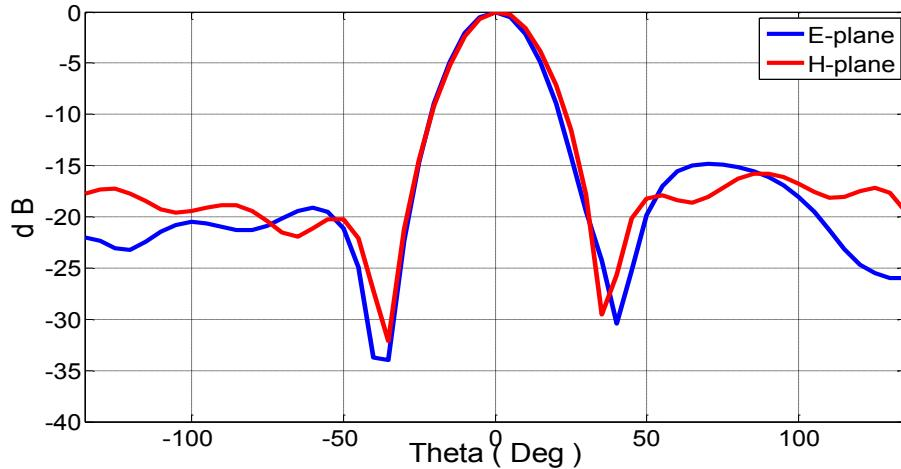
Figure 3.3: E- and H-plane radiation patterns of the simulated  $2 \times 2$  DD patch antenna array with a conventional superstrate [93].
