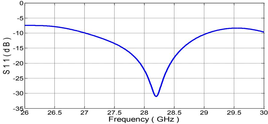
Figure 3.2: Reflection coefficient of the simulated  $2 \times 2$  DD patch antenna array with a conventional superstrate [93].
