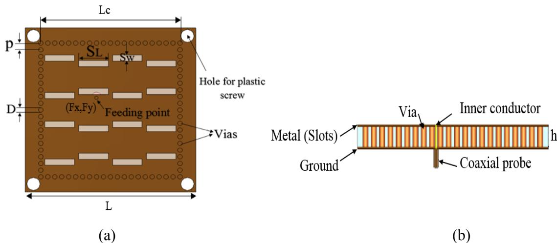
Figure 6.1: Geometry of the proposed antenna: (a) top view; (b) side view [71].
