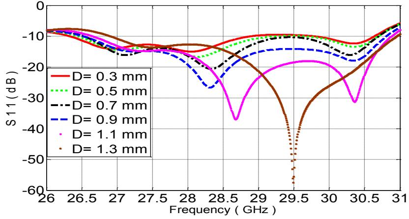
Figure 3.6: Simulated reflection coefficient of the antenna considering the effect of varying the diameter of the holes on the superstrate layer [93].
