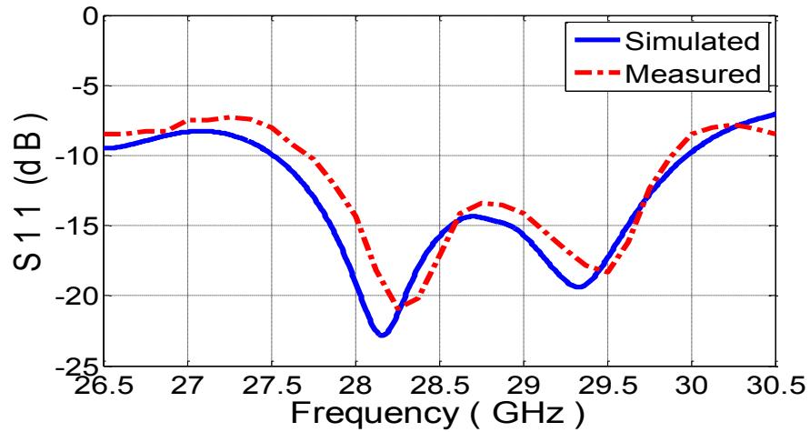
Figure 5.4: Reflection coefficient of the DD patch antenna with a positive reflection phase unit cell [91].
