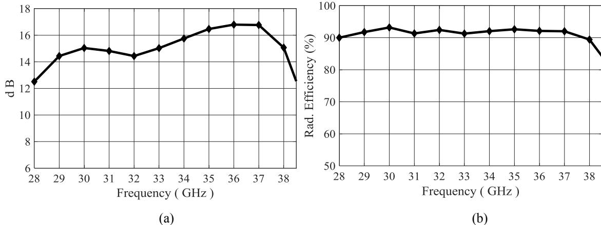
Figure 3.18: Simulated gain (a), and radiation efficiency (b) of the proposed antenna with a thin PRS superstrate.
