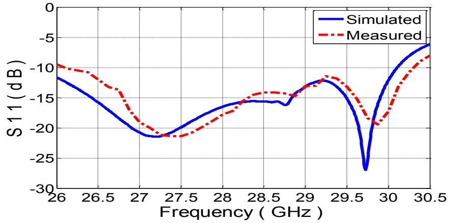
Figure 5.12: Reflection coefficient of the DD patch antenna with a positive reflection phase superstrate [91].
