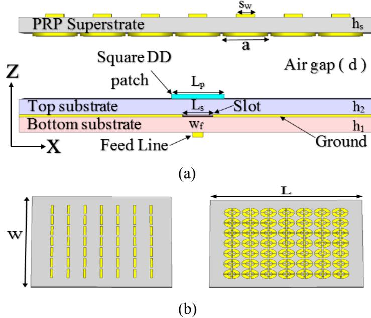
Figure 5.11: Geometry of the proposed antenna with PRP unit cells: (a) side view, (b) top and bottom of the superstrate [91].
