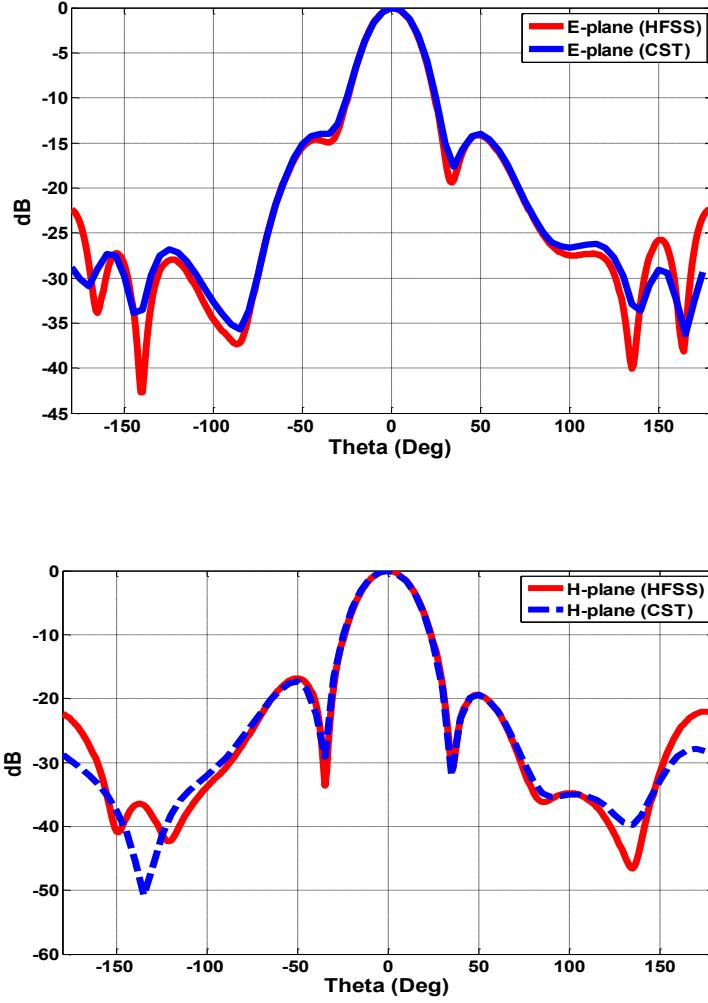
Figure 6.4: The E- and H-plane radiation patterns of the LP SIW cavity antenna [71].
