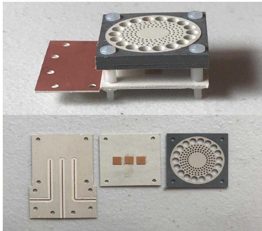
Figure 4.8: Photograph of the proposed antenna with tapered superstrate for a beam tilting antenna.
