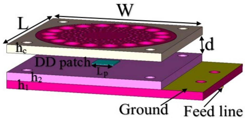
Figure 4.2: Geometry of the proposed antenna: side view.
