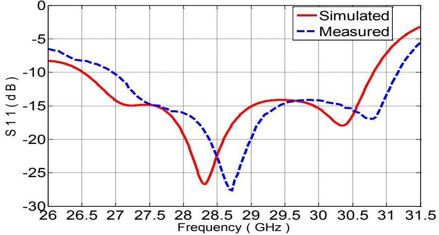
Figure 3.8: Measured and simulated reflection coefficients of the proposed antenna [93].
