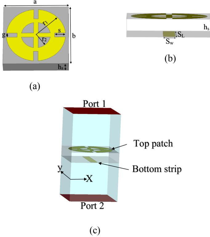
Figure 5.7: Geometry of the proposed unit cell: (a) top view, (b) side view, and (c) characterization model of the unit cell [91].
