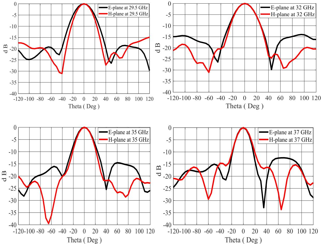
Figure 3.19: E and H-plane radiation patterns of the proposed antenna with a thin PRS superstrate at different frequencies.
