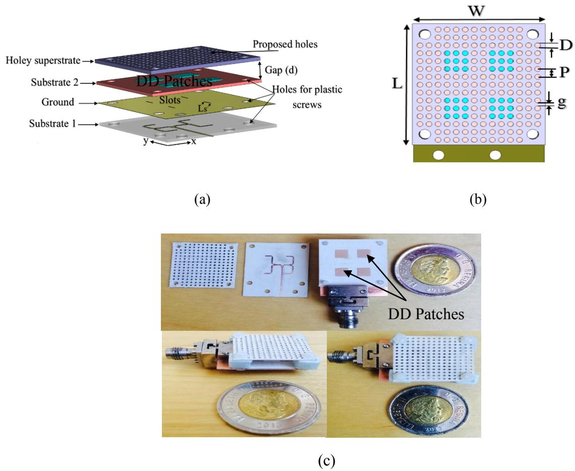
Figure 3.4: Geometry of the proposed antenna: (a) side view, (b) top view, and (c) photographs of the antenna prototype [93].
