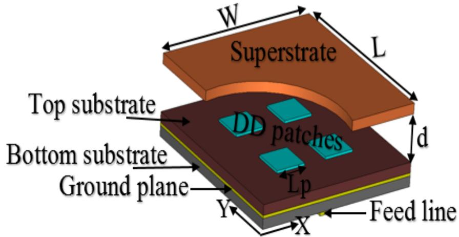
Figure 3.1: Geometry of the  $2\times 2$  DD patch antenna array: side view. Superstrate is partly removed to show the patches under it [93].
