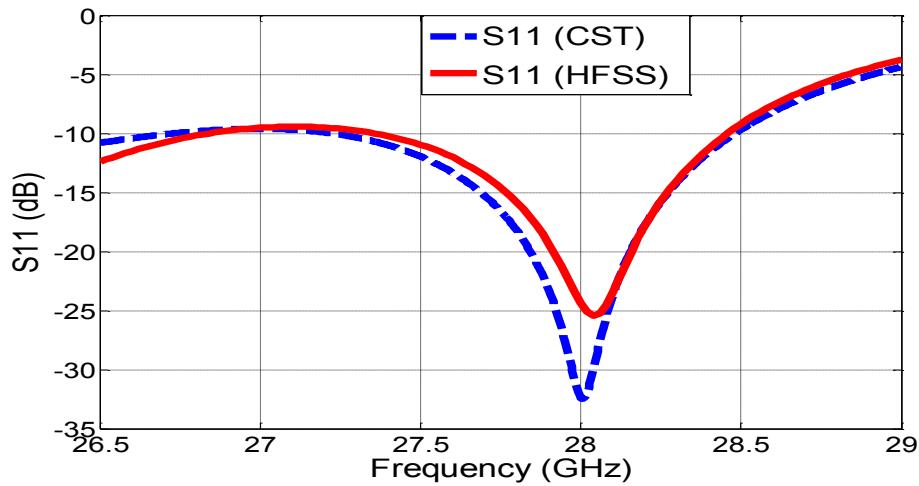
Figure 6.2: Simulated reflection coefficient of the LP SIW cavity antenna [71].
