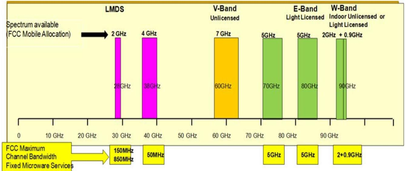
Figure 1.4: potential 5G spectrum above 20 GHz [5].
