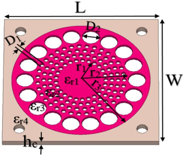
Figure 4.1: The geometry of the proposed tapered superstrate.
