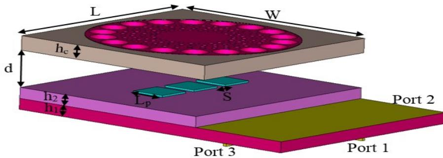
Figure 4.7: Side view of the proposed antenna with three ports for beam tilting.
