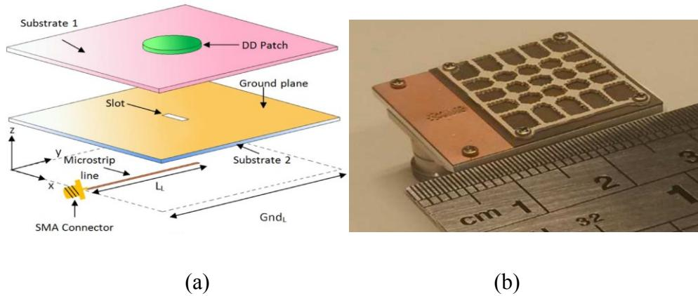
Figure 1.5: A single DD patch [24] (a), planar DD patch array [25] (b).
