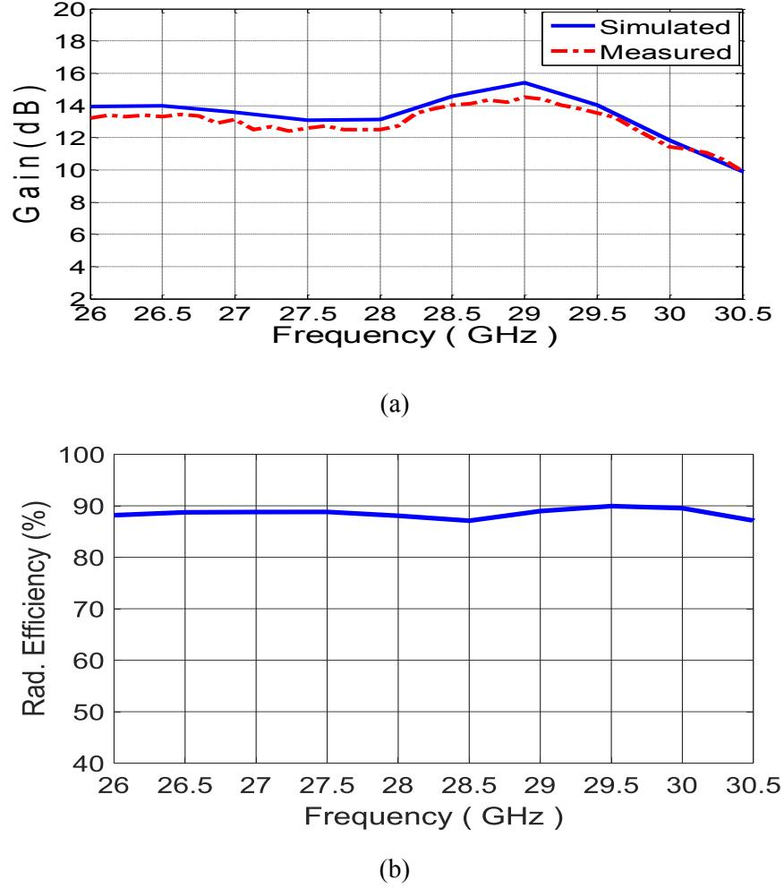
Figure 5.13: Gain (a) and radiation efficiency (b) of the DD patch antenna with a positive phase gradient unit cell [91].
