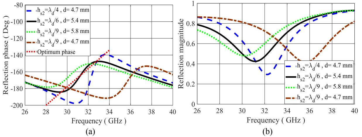
Figure 3.15: Effect of changing the bottom substrate thickness of the proposed unit cell on the PRS performance: reflection phase (a), and reflection magnitude (b).
