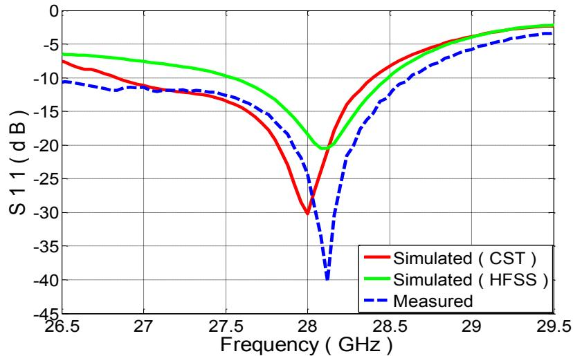
Figure 6.10: Simulated and measured reflection coefficient of the proposed CP SIW cavity antenna [71].
