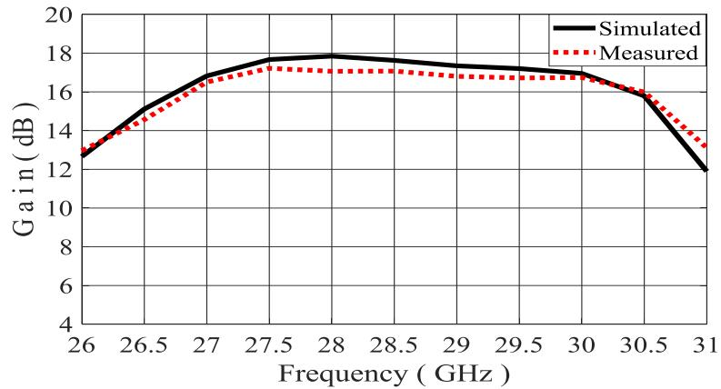
Figure 4.5: Measured and simulated gain of the implemented antenna.
