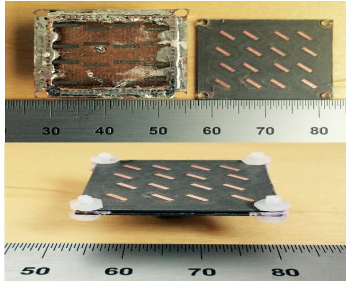
Figure 6.7: Prototype of the fabricated CP SIW cavity antenna. (a) Top of the antenna and convertor, and (b) side view [71].
