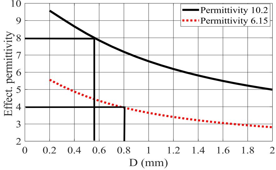
Figure 3.13: Calculated effective permittivity of the PRS slabs.
