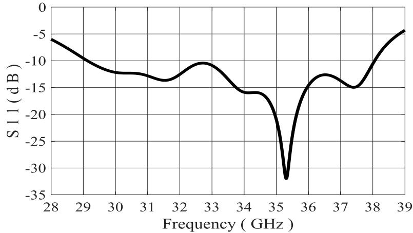
Figure 3.17: Simulated reflection coefficient of the proposed antenna with a thin PRS superstrate.
