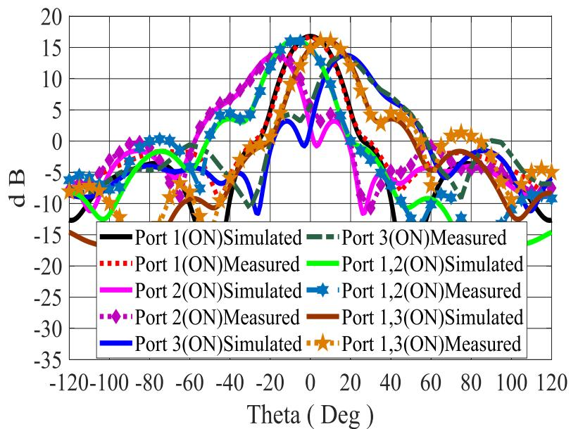
Figure 4.11: Simulated and Measured H-plane radiation patterns.
