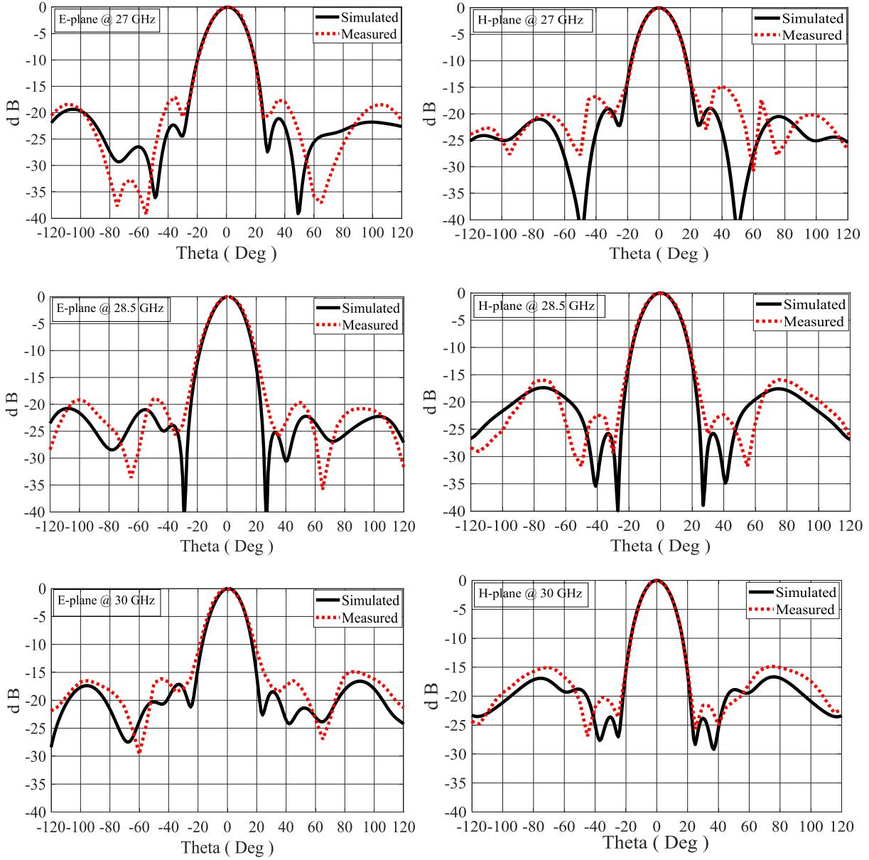
Figure 4.6: Measured and simulated E and H-plane radiation patterns of the proposed antenna at different frequencies.
