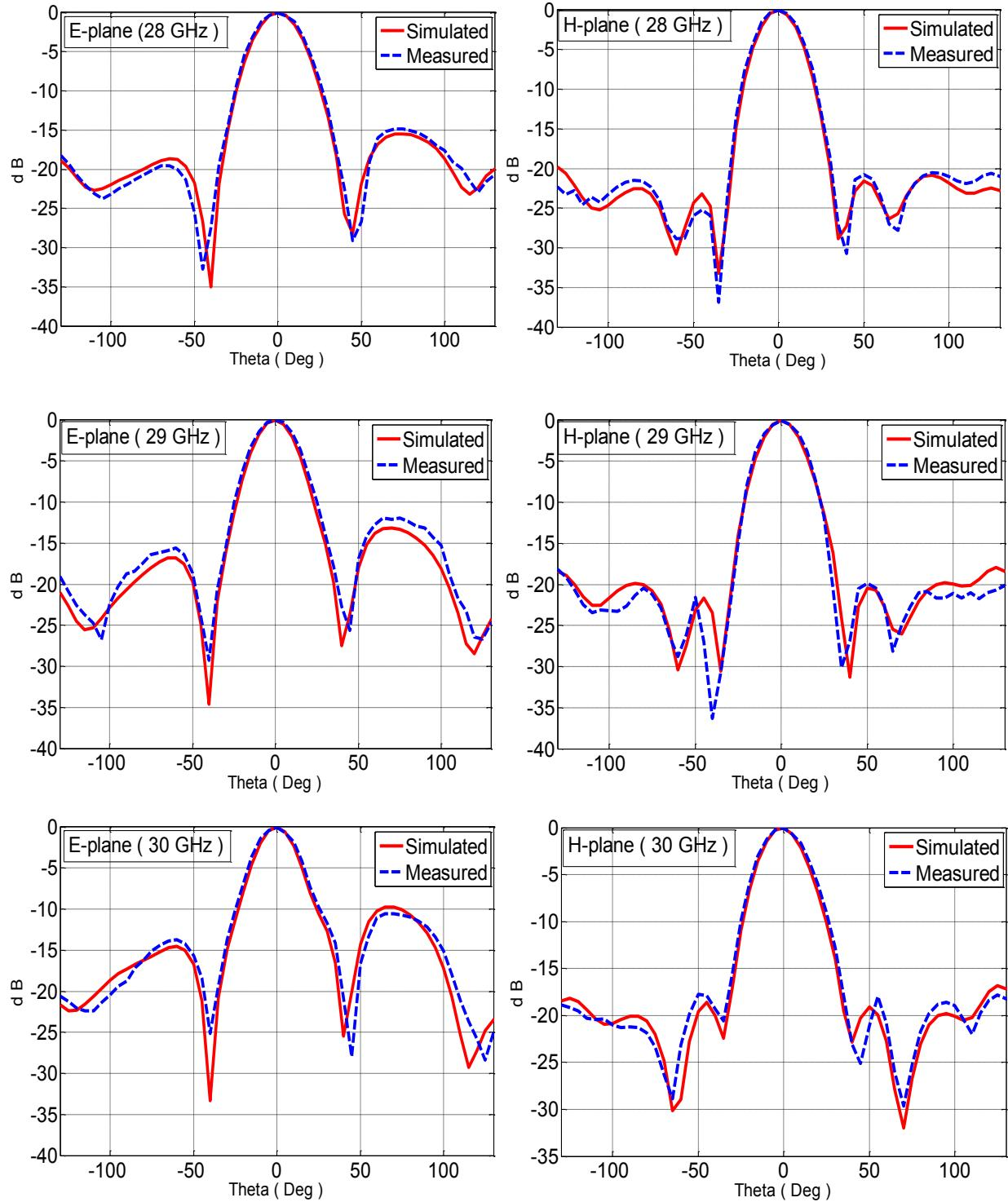
Figure 3.11: Simulated and measured radiation patterns of the DD patch antenna array with a perforated superstrate [93].
