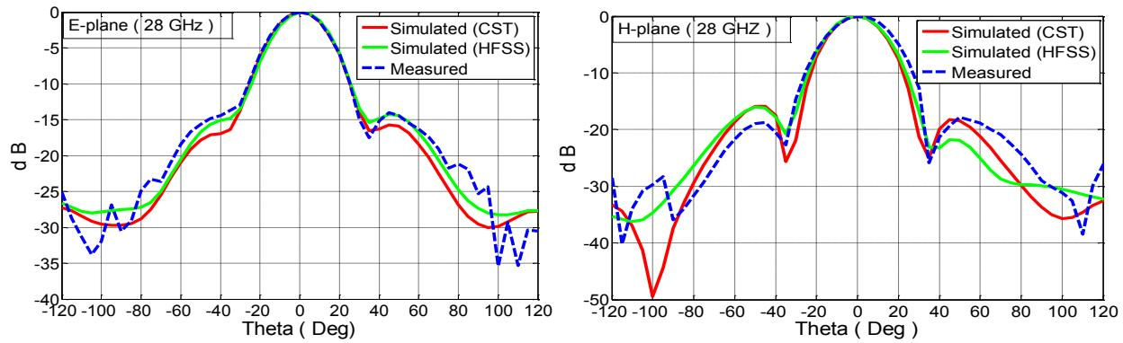
Figure 6.12: Radiation pattern of the proposed CP SIW cavity antenna [71].
