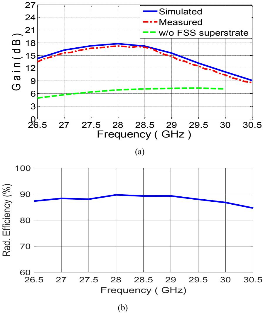
Figure 5.5: Simulated and measured gain (a), and simulated radiation efficiency (b) of the proposed antenna [91].
