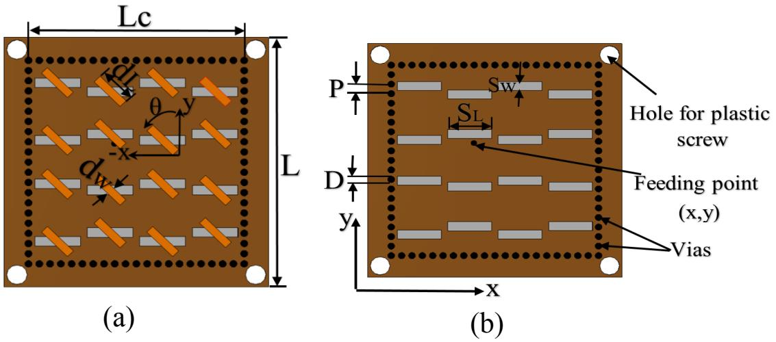
Figure 6.5: Geometry of the proposed CP SIW cavity antenna: (a) top view of the converter, (b) top view of the slotted SIW cavity, and (c) side view [71].
