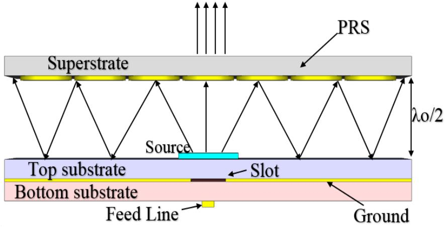
Figure 1.6 Schematic diagram of a PRS Fabry Perot Cavity antenna [109].
