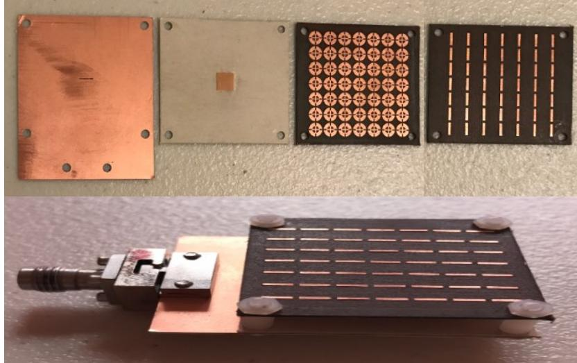
Figure 5.16: The prototype of the proposed antenna [91].
