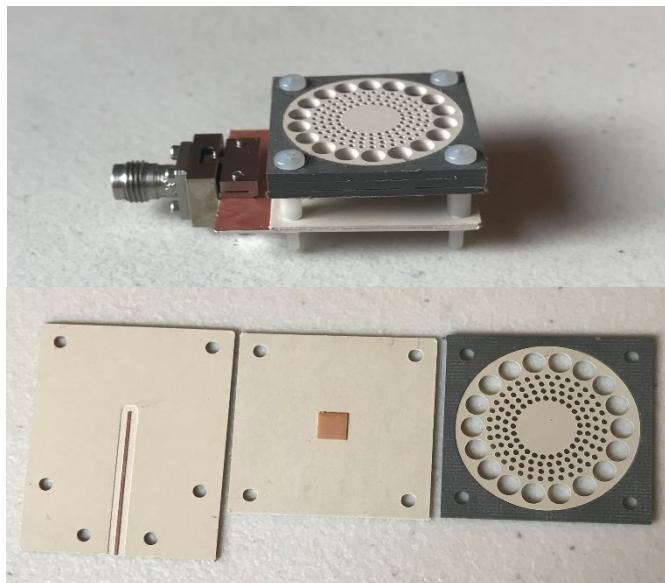
Figure 4.3: A photograph of the proposed antenna prototype.
