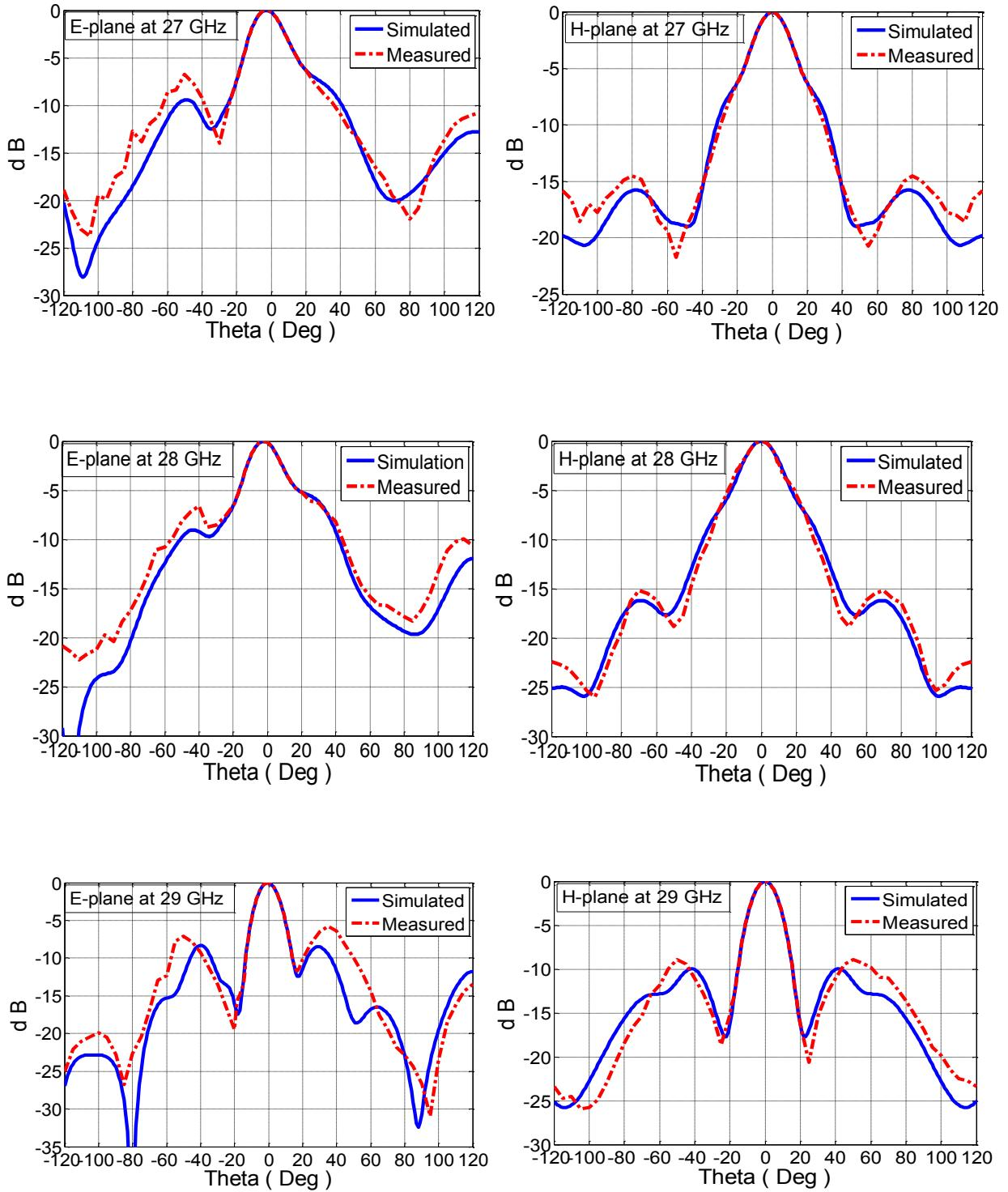
Figure 5.15: E- and H-plane radiation pattern of the DD patch with a positive phase superstrate at four different frequencies [91].
