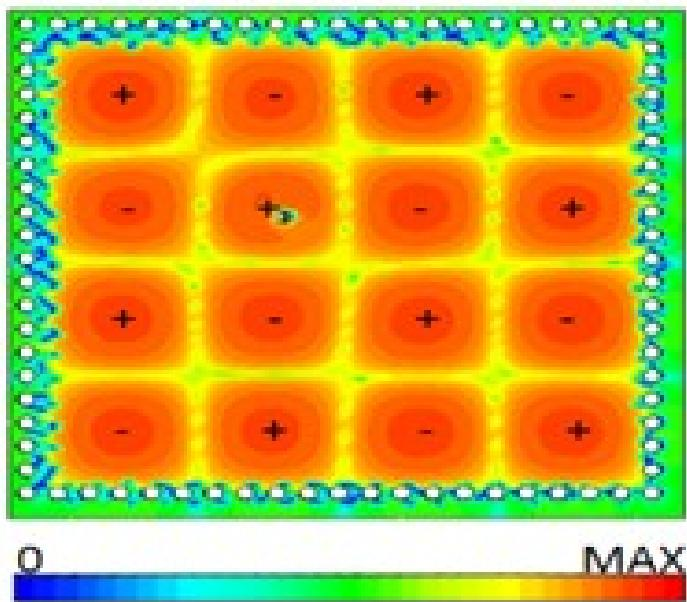
Figure 6.6: Distribution of the magnitude of the E-field for the TE440 mode at 28 GHz inside the CP SIW cavity [71].
