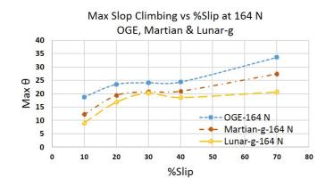
Figure 4.31: Ability of the rover to climb slopes at 164 N wheel loading, slip 10-70% in Partial gravity and OGE
