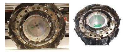
Figure 2.1: A prototype of the innovative ExoMars flexible wheel
