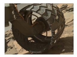
Figure 1.2: Punctures in the Curiosity rover wheel reduce rover mobility. Image credit: NASA/JPL-Caltech
