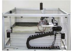
(c) Single-wheel testbed developed by CMU [53]
