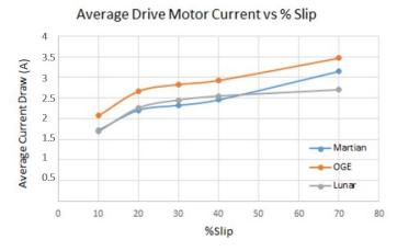
Figure 4.34: Average current draw from wheel motor vs %slip at 164 N wheel loading
