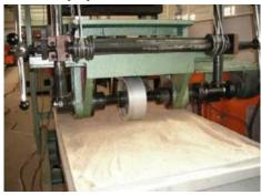
(d) Single-wheel testbed developed by Jilin University [35]
