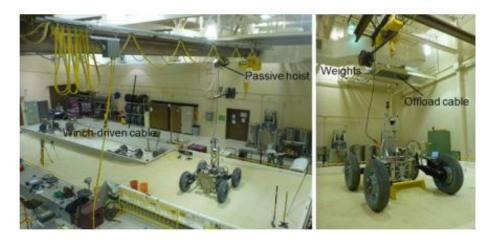
Figure 1.13: Gravity offloaded excavation experiments at NASA Glenn Research Centers (GRC) Simulated Lunar OPErations (SLOPE) lab. A cable pulls up on the robot, tensioned by weights acting through a lever arm. The offload assembly hangs from a hoist that is pulled along a rail by a separate winch-driven cable, as marked [55].
