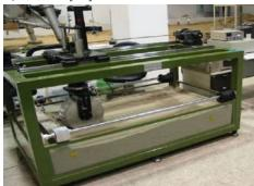
(e) Single-wheel testbed developed by HIT [22]
