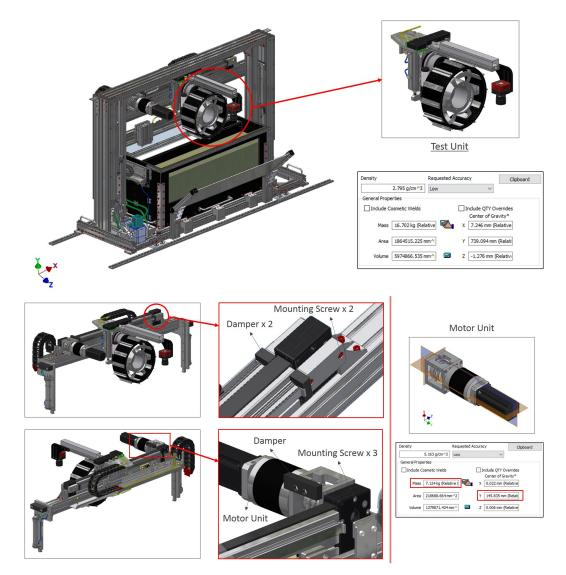
Figure A.40: Test item unit capture and damping hardware
