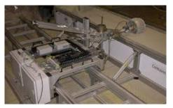
(b) Single-wheel testbed developed by DLR [38]
