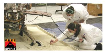
Figure 1.3: Sandbox setup at NASA's Jet Propulsion Laboratory, Pasadena, Calif., where engineers used a 3/8 mass test rover to assess possible moves for getting Mars rover Spirit out of a patch of loose Martian soil. Image credit: NASA/JPL-Caltech
