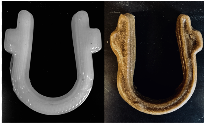
Figure 43: Simple gripper fabricated using DIW 3D printing method.
