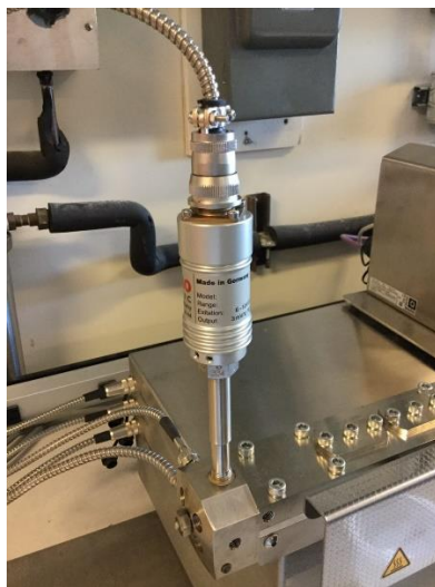
Figure 3.9 Different parts of twin-screw extruder: The pressure sensor (Left) and controller (Right)
