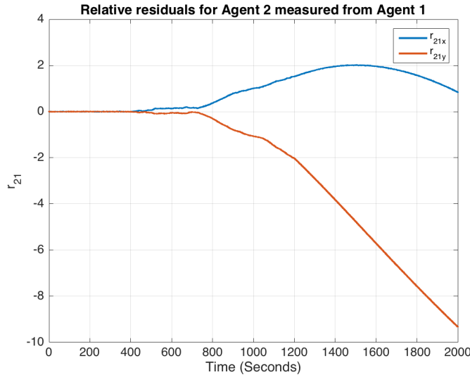
Figure 3.28: Relative residuals for Agent 2 measured from Agent 1 when Agent 2 is under an attack.
