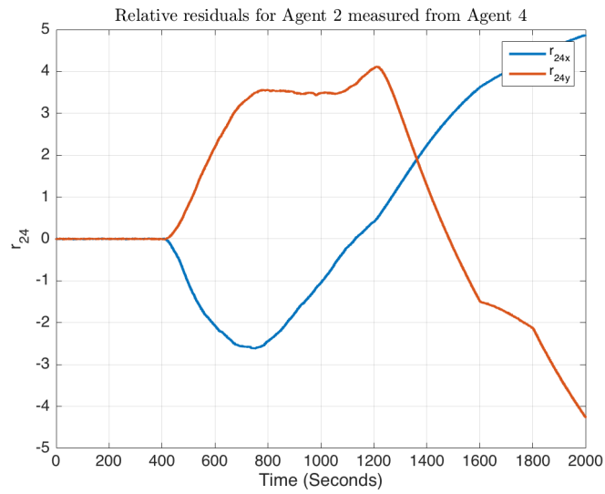
Figure 3.36: Relative residual signals for Agent 2 measured from Agent 4 when the team is under attacks and faults.
