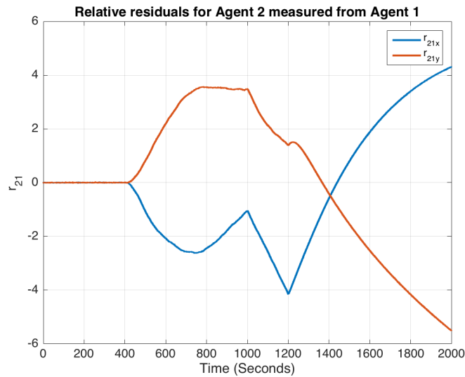
Figure 3.35: Relative residuals for Agent 2 measured from Agent 1 when the team under attack and fault.
