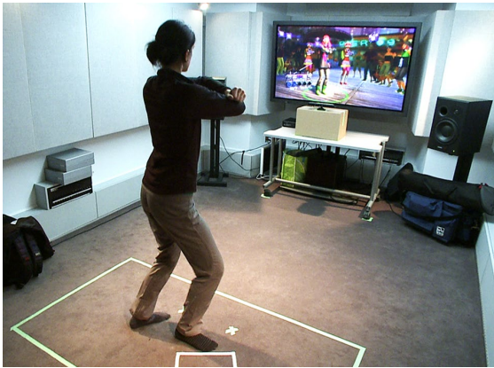
Fig. 1 Dance imitation task. The participants stand facing the television screen where they view an avatar dancing using whole-body movements, and are asked to mirror the avatar's movements in real time. Participants' movements are registered by the Kinect sensor
