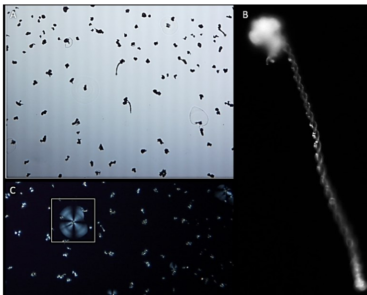
Figure 16. Silica-carbonate microstructures grown in non-degassed aqueous solutions of \text{BaCl}_2 (19 mM) and \text{Na}_2\text{SiO}_3 (8.2–8.5 mM), where the former was added to the latter in a 100 mL beaker. The total solution volume was 15 mL, and was adjusted to pH 11.2, prior to the addition of fluorescein dye (1.40 mM). The material precipitated on a clean microscope slide positioned vertically in solution, while a petri dish was used to cover and allow the flow of \text{CO}_2 in through the spout of the reaction vessel. After ca. two hours, the slide was removed and rinsed twice in distilled water, followed by acetone and finally air dried prior to the morphological characterization of the shapes: A) optical light micrograph showing the morphologies (pH 11.2); B) translucent double helix viewed by dark field optical microscopy; and C) a leaf-like shape displaying a dark extinction pattern when viewed between crossed polarizers of a petrographic microscope.
