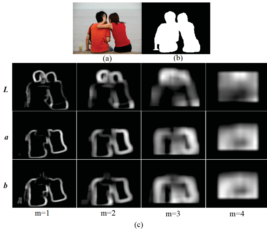
Figure 4.1: (a) A sample image, (b) the corresponding ground truth, and (c) local feature maps obtained after m = 1, 2, 3, 4 level of NSCT decomposition for the L , a and b color channels.
