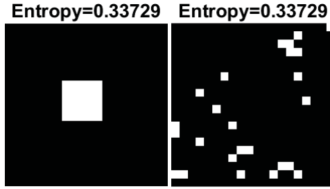
Figure 3.3: Synthetic images of size 20 \times 20 pixels, each of two images has 25 pixels with the gray level of 1 and 375 pixels with the gray level of 0.
