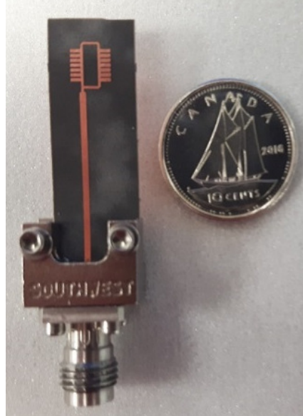
Figure 2.1.18: Proposed wideband antenna structure actual prototype.
