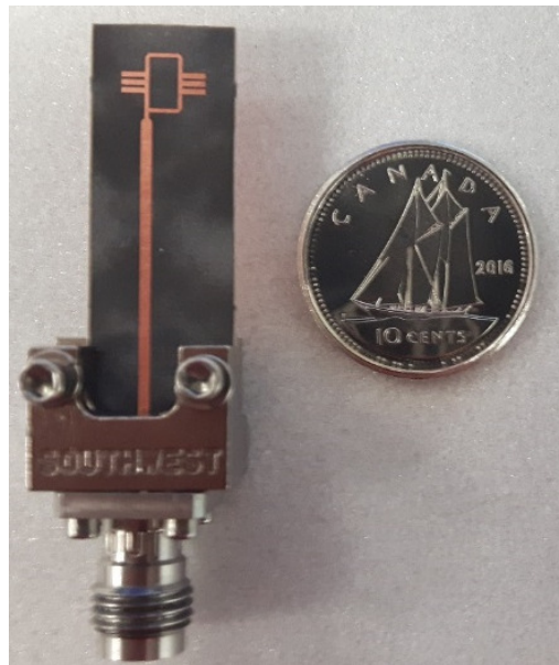
Figure 2.1.12: Photo of the proposed narrowband antenna, the microstrip line feed length is 21 mm.
