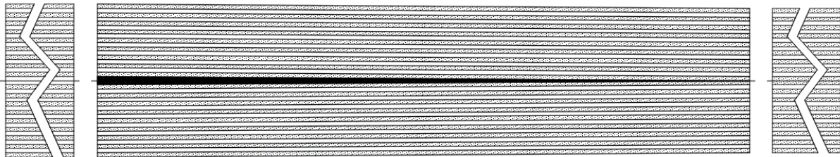
Figure 2.5 Step 1: 2 plies dropped-off
