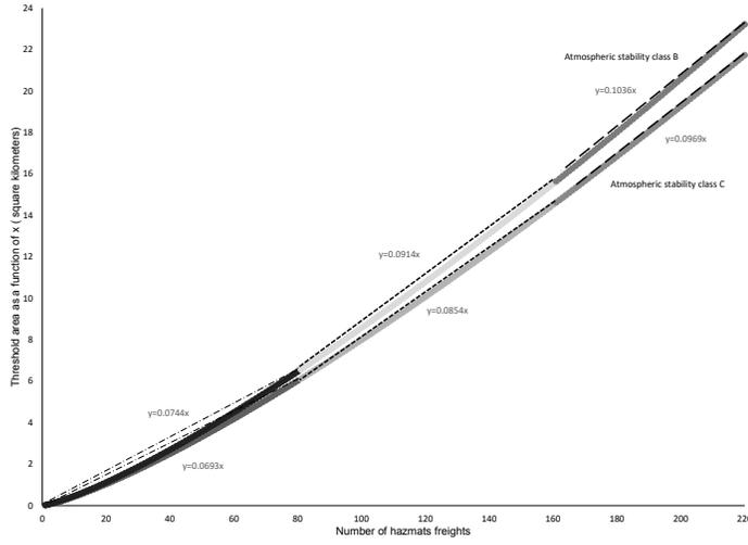
Figure 2.3: Piecewise linearization for threshold area.
