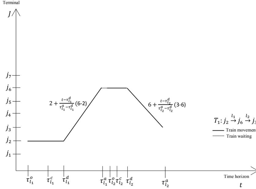
Figure 4.3: An example of string-line diagram.
