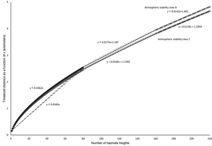
Figure 2.2: Piecewise linearization for threshold distance.
