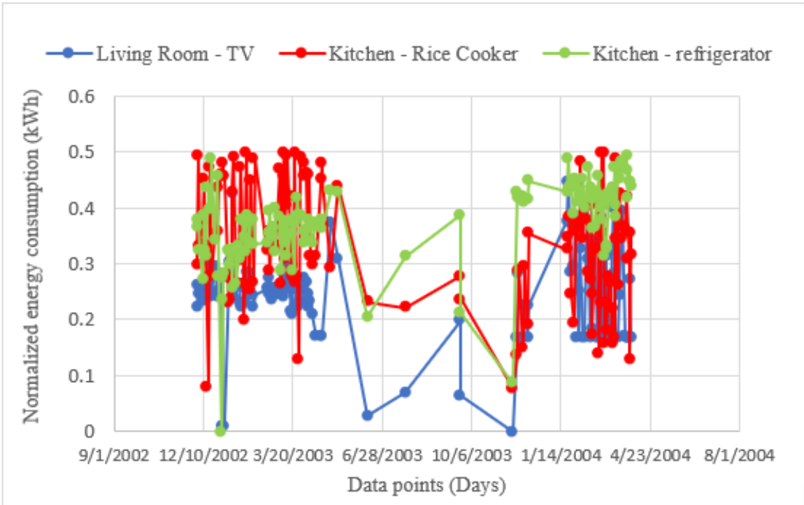
Figure 3-9. Normalized energy consumption of end-use loads based on rule 1. The upper and lower figures show the inputs and output of the ANN model. The data points are extracted from the dataset and are not successive days. Also, the days come from the same cluster.
