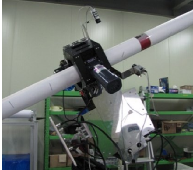
FIGURE 2-2 BRIDGE CABLE INSPECTION ROBOT- RESEARCH PROJECT
