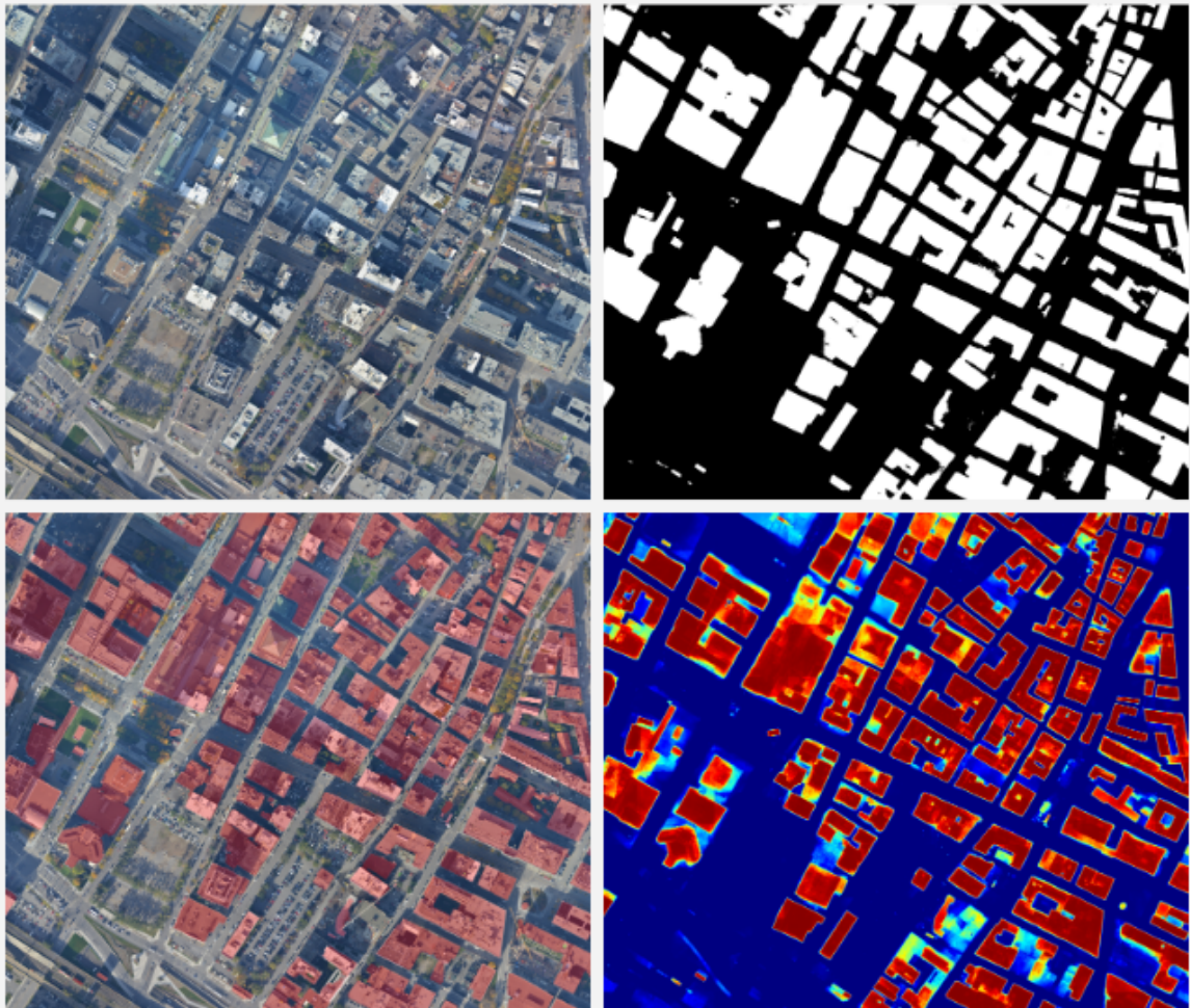
Figure 5.1: Building Classification of Montreal data. Top left: The orthophoto RGB input image. Bottom left: The prediction of ICT-Net overlaid on top of the RGB image(Red-Prediction). Bottom right: The probability mask of ICT-Net shown as a heat map. Top right: The binary segmentation map resulting after the thresholding of the raw ICT-Net output. The orthophoto RGB image is courtesy of Defence Research and Development Canada and Thales Canada.
