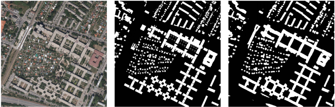
Figure 3.2: Building Classification of a patch from vienna city, tile 02. Result for an image from the validation dataset. Left: A patch from vienna city as input image. Middle: The semantically labeled ground truth image. Right: The binary map prediction resulting after the thresholding of the probability output from the capsule based segmentation network.
