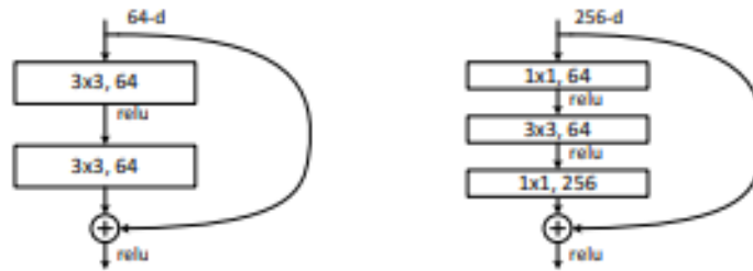
Figure 2.4: An illustration of the 2 different types of ResNet [21] block. Left: a ResNet building block for ResNet34. Right: a “bottleneck” ResNet building block for ResNet-50/101/152
