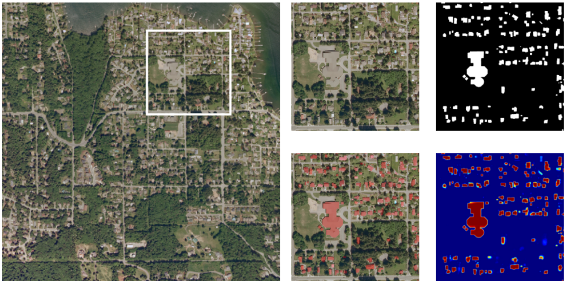
Figure 4.4: Building Classification of Bellingham city, tile 17. Result for an image from the test dataset. Top left: A closeup of a small area of an input image. Bottom left: The probability image overlaid on top of the RGB image. Bottom right: The probability image shown as a heat map. Top right: The binary map resulting after the thresholding of the probability image.
