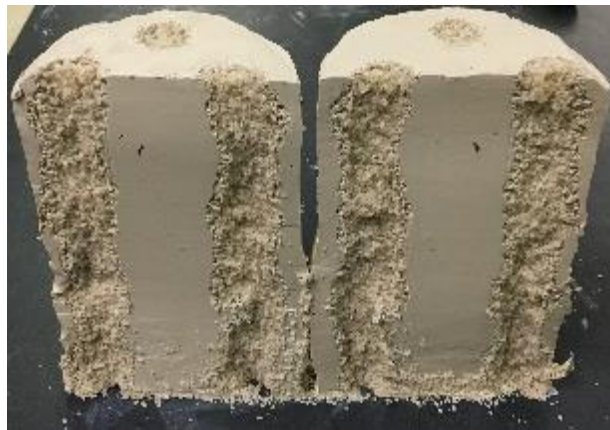
(c) bending failure (CTS 7, T2)
