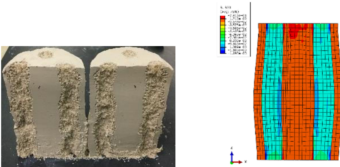
(c) Bending failure (CTS 7, T2)
