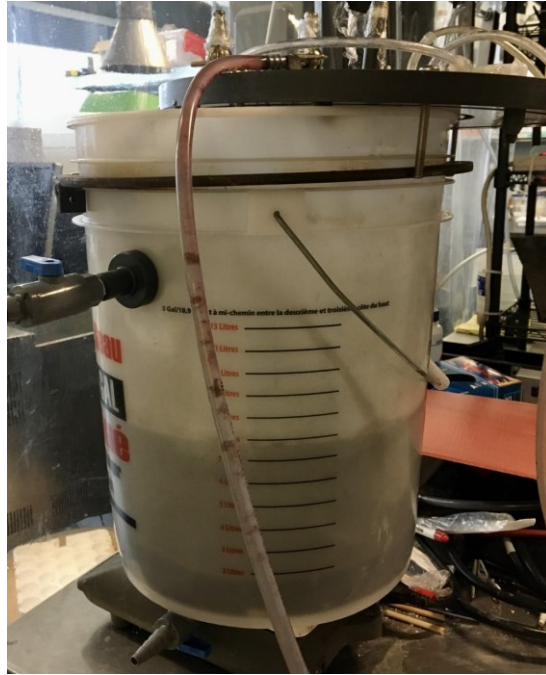
Figure 7: Bucket used for reactors
