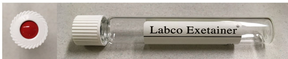
Figure 13: Vials and special caps used for gas sampling
