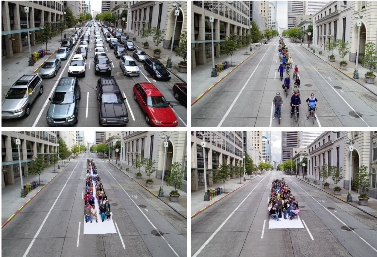
Figure 1: “The Commuter Toolkit” poster (edited) 200 people commuting in 177 cars (upper left), their bikes (upper right), 3 buses (bottom left) or one light rail train (bottom right). Produced by International Sustainable Solutions (ISS) for the International Sustainability Institute (ISI) (i-SUSTAIN, 2008; Rivenburgh & Chase, Patricia, 2019)
