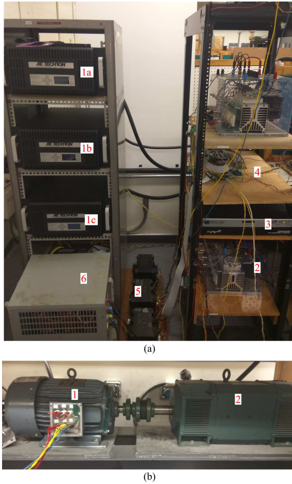
Fig. 3.9: (a) Experimental setup of the emulator system (1) Linear amplifiers emulating the VFM (2) Driving inverter (3) Controller for the VFM emulator (4) protection circuitry (5) link inductors and (6) isolation transformer; (b) Experimental setup of the VFM drive (1) The VFM machine (2) coupled DC dynamometer.
